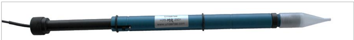
Figure 3: H 2 S sensor in the Microrespiration guide.
