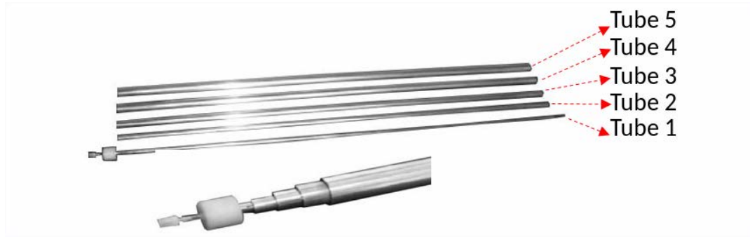
FIGURE 4.6 – Sensitivity phantom used for experiments and modelled for simulations.
