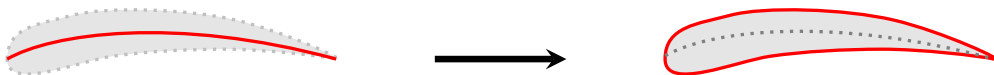
FIGURE 2.1: Reverting from the simplified mean camber zero-thickness surface representation of turbine blades to a three-dimensional full-thickness rendition.
