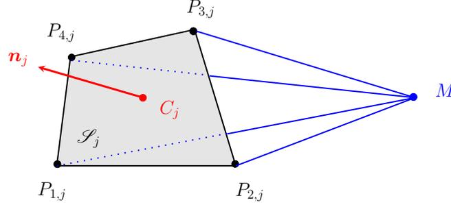
**FIGURE 2.6:** Schematic representation of a quadrangular mesh face  $\mathcal{S}_j$  of normal  $\mathbf{n}_j$  and center  $C_j$  and the quantities necessary for the computation of the velocity potential at the evaluation point  $M$  of coordinates  $\mathbf{x}$ .
