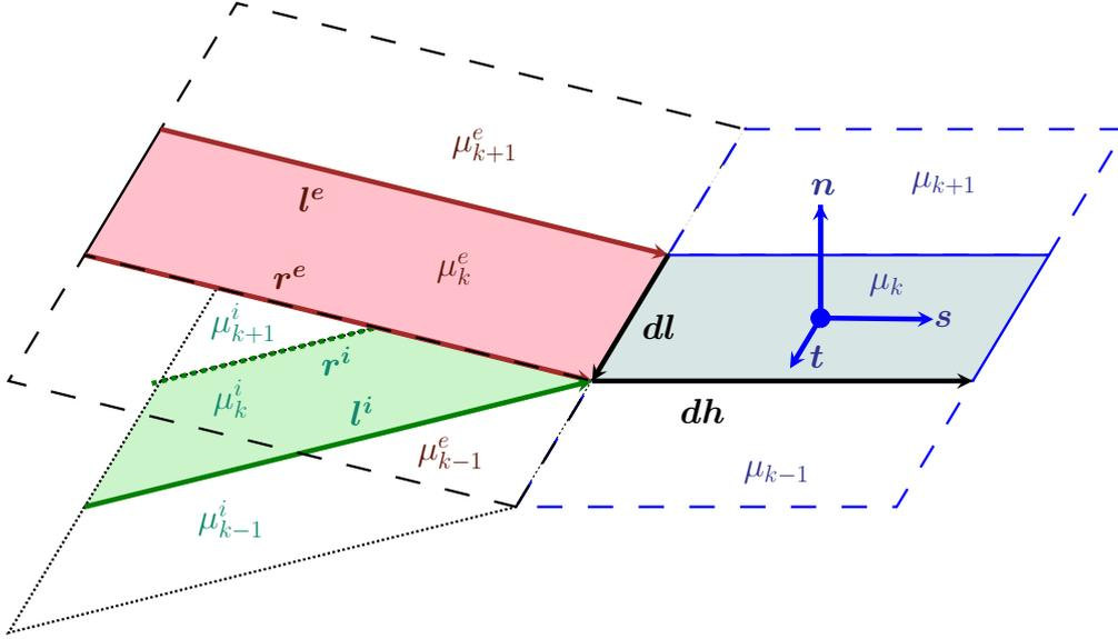
**FIGURE 2.5:** Schematic representation of a thick blade trailing edge : extrados and intrados faces along the trailing edge, with their left and right hand neighbor faces, and the dummy faces following the trailing edge at the onset of the wake.
