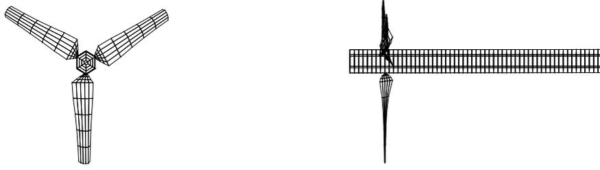
**FIGURE 1.2:** Example of discretisation of a three-bladed horizontal axis tidal turbine into a zero-thickness quadrangular surface mesh.
