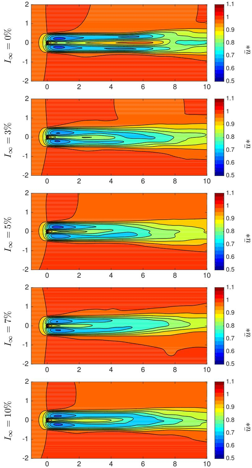
**FIGURE 4.7:** Time-average of one turbine wake with various ambient turbulence intensities (with no hub and no mast) : Poletto's DFSEM turbulence filtered,  $TSR = 2.5$ ,  $U_\infty = 1.0$ ,  $R_f = 1$ ,  $\lambda = 0.5$ ,  $\sigma(\lambda) = 0\%$ ,  $(\sigma_u : \sigma_v : \sigma_w) = (1.0 : 1.0 : 1.0)$ .
