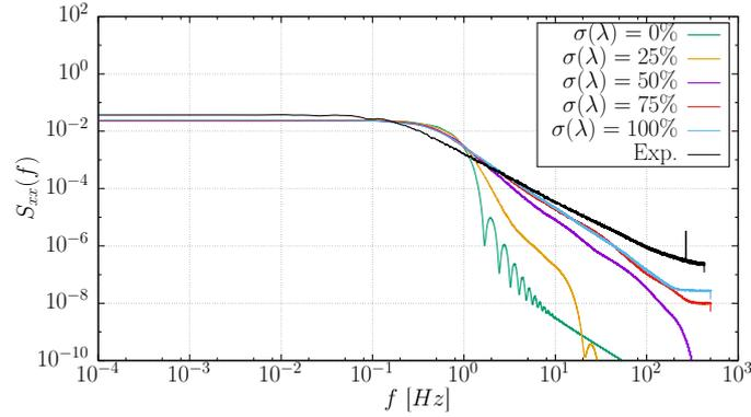
**FIGURE 3.15:** Influence of  $\sigma(\lambda)$  on the spectral representation for a Gaussian kernel ( $\lambda = 0.5$  and  $R_f = 2$ ) and comparison with experimental data provided by Medina et al. [102] (for  $I_\infty = 15\%$  and  $U_\infty = 0.8$  m/s).
