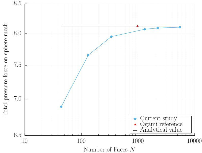
**FIGURE 2.16:** Value of the total pressure force on the unmoving sphere mesh in an accelerated flow, using increasingly refined meshes, compared to the analytical value and the result obtained by Ogami.
