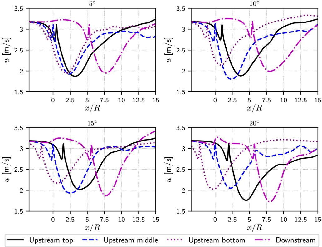
**FIGURE 5.13:** Time-averaged wake lines obtained for four yaw angles ( $I_\infty = 10\%$ ,  $L = 18$  m,  $Rf \approx 229$ ,  $TSR=4.1$ ,  $\sigma(\lambda) = 75\%$ ). For each turbine, the corresponding line passes through its centre.
