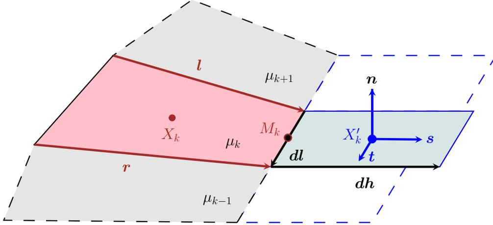
**FIGURE 1.5:** Schematic representation of the emission of an imaginary wake mesh face  $\mathcal{S}'_k$  behind the trailing edge mesh face  $\mathcal{S}_k$ .
