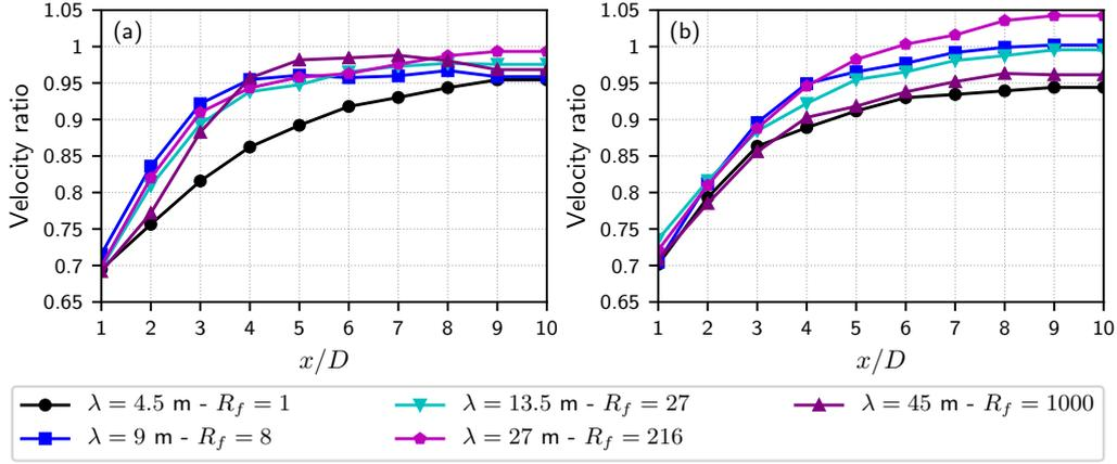
FIGURE 5.7: Comparison of the numerical disc-averaged velocities obtained for  $TSR=4.1$ ,  $I_\infty=10\%$  and several  $\lambda$ . (a)  $\sigma(\lambda) = 0\%$ . (b)  $\sigma(\lambda) = 75\%$ .
