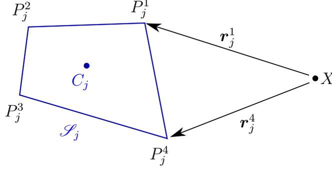
**FIGURE 1.3:** Schematic representation of a mesh face  $\mathcal{S}_j$  showing the notations used to compute its interaction with a distant point  $X$ .
