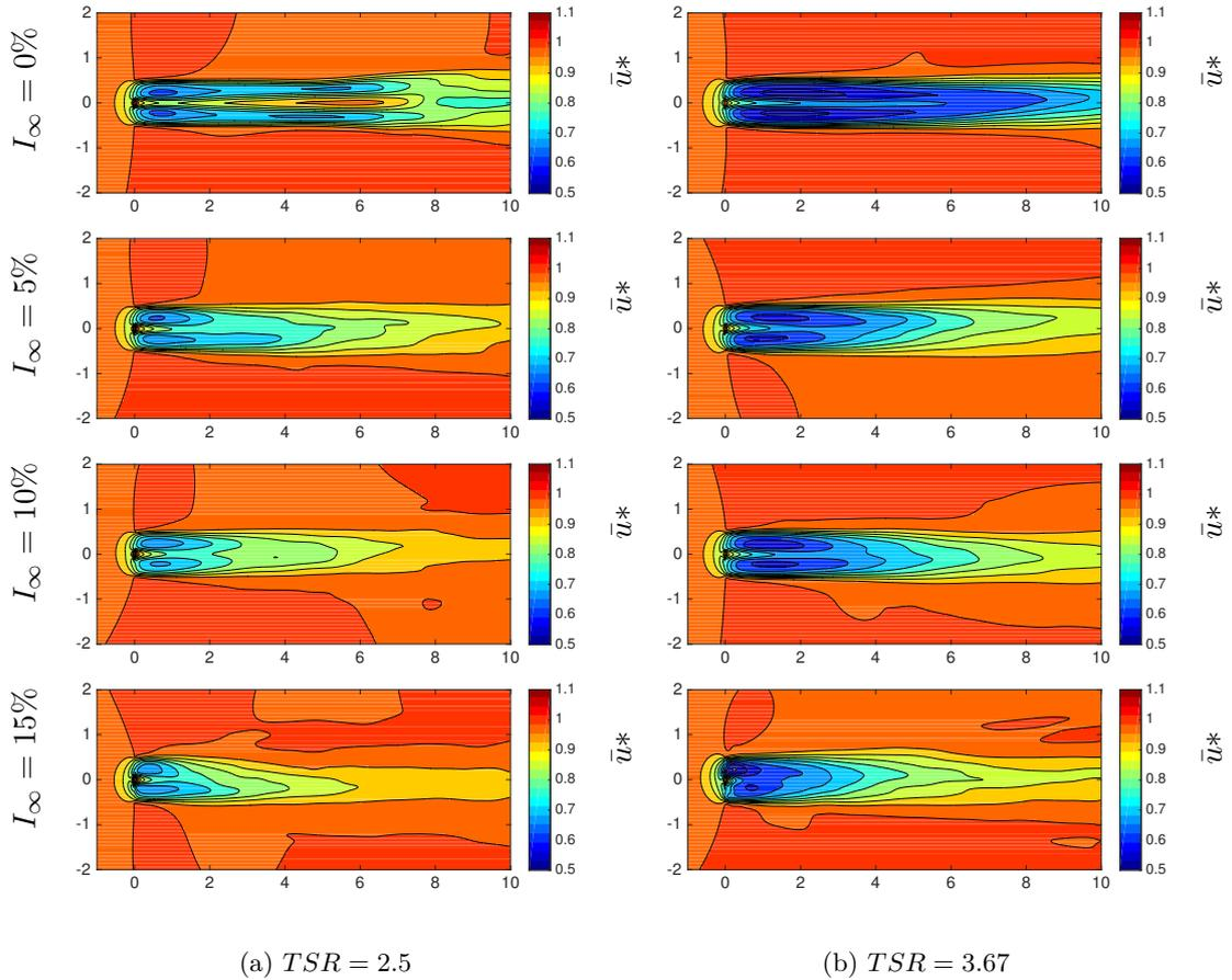
**FIGURE 3.18:** Velocity maps in the wake of a single turbine, averaged over a period of 50 to 80 seconds, for varying levels of turbulent intensity. The  $x$  and  $y$  axis were made dimensionless with respect to the turbine diameter  $D$ .  $\bar{u}^*$  stands for the dimensionless velocity field and is defined as  $|\bar{u}|/U_\infty$ .
