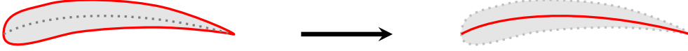
FIGURE 1.1: Schematic representation of the passage from the "true" thick geometry of a turbine blade to the thin profile mean camber surface used in the simulations carried out with the Dorothy simulation code.
