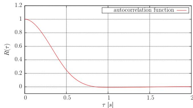
**FIGURE 3.16:** Sample plot of an autocorrelation function  $R(\tau)$  calculated with the numerically generated velocity field
