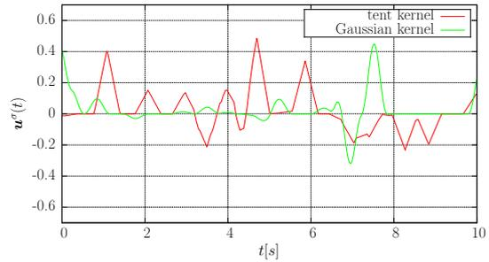
**FIGURE 3.12:** Temporal measurements of velocity fluctuations  $u^\sigma(t)$  at one point, for different kernel functions  $f_\lambda$  (with  $I_\infty = 15\%$ ,  $\lambda = 0.25$ ,  $\sigma(\lambda) = 25\%$ ,  $R_f = 1$ ).
