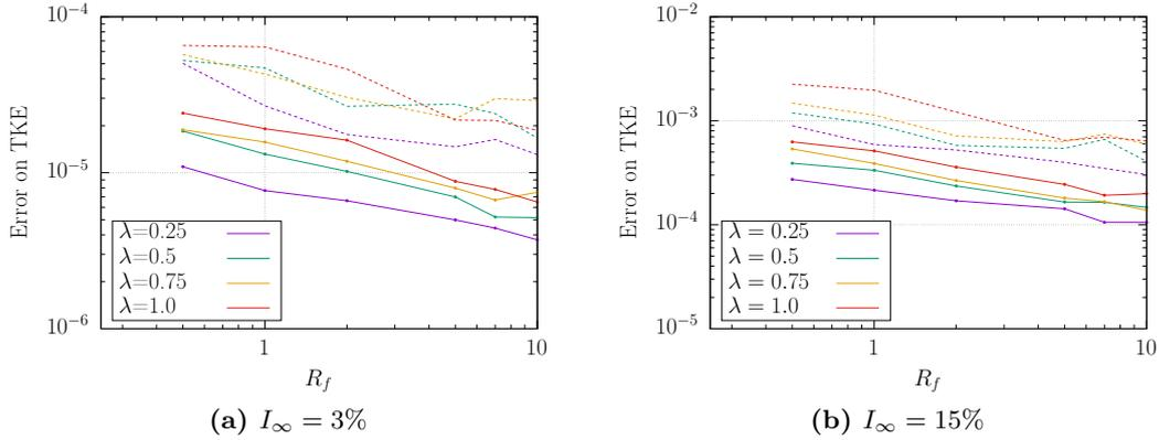
**FIGURE 3.9:** Average error (full lines) and maximal error (dashed lines) on the value of the TKE  $K$  plotted against the filling ratio  $R_f$ , for various size of turbulent structures  $\lambda$ . For both the cases of low turbulence intensity (a) and high turbulence intensity (b) :  $\sigma(\lambda) = 0\%$ , and the sub-function  $f_\lambda$  uses the Gaussian kernel.
