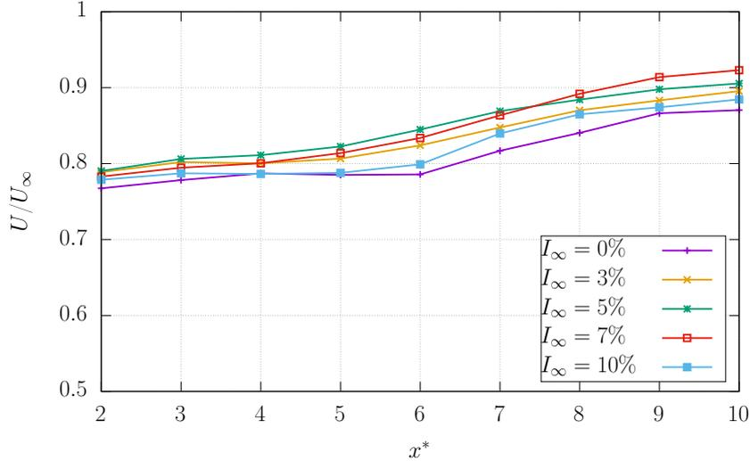
**FIGURE 4.8:** Velocity ratio  $u/u_\infty$  integrated in the wakes of the turbine blades shown in Figure 4.7, using varying levels of turbulence intensity  $I_\infty$  generated with Poletto’s DFSEM.
