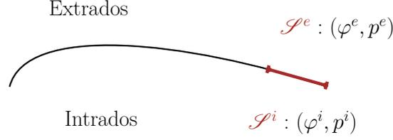
**FIGURE 1.4:** Schematic representation of a thin blade profile showing both sides of its trailing edge mesh face.
