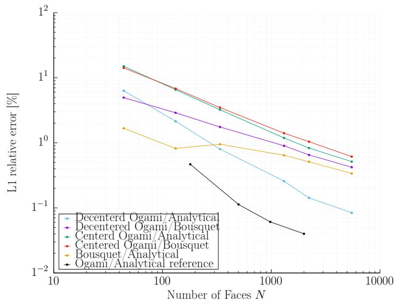
**FIGURE 2.12:**  $L_1$  errors between different version of potential calculations on increasingly refined sphere meshes, relative to upstream velocity  $U_\infty$ , compared to the results given by Ogami [86].
