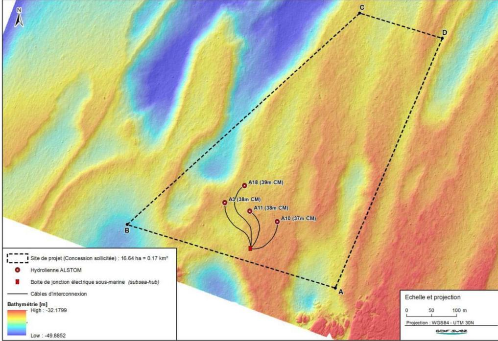
**FIGURE 5.1:** Configuration of the NEPTHYD project : a four turbine pre-commercial farm developed by Engie in 2014 and meant to be equipped with Alstom’s Oceade™ turbine. The image is reproduced from the report [105] of the Autorité Environnementale, an agency of the French Ministry of Energy and Environment.
