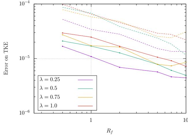
**FIGURE 4.4:** Maximal (dotted lines) and average (full lines) errors committed on the Turbulent Kinetic Energy depending on the size of the turbulent structures used (averaged using 50 sample times series of 6 hours each for each set of parameters).
