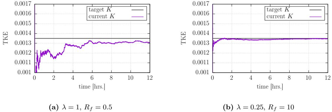
**FIGURE 3.8:** Time series of the current values of the TKE  $K$  computed at a single point over 12 hours of simulated time, for the low turbulence intensity  $I_\infty = 3\%$ . On the left : an example of very slow convergence, with few turbulent structures of large size  $\lambda$ . On the right : an example of fast convergence, with a high saturation  $R_f$  of structures of small size  $\lambda$ .
