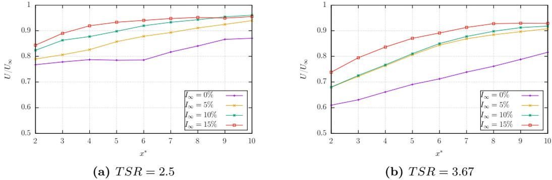
**FIGURE 3.19:** Velocity integrated in the wake of a single turbine, on a disc of the same width as the turbine and at given distances downstream of its centre. These curves are produced using the numerical wake velocities shown in map form in the previous Figure.
