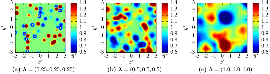
**FIGURE 3.5:** Example of velocity fields provided by the Synthetic Eddy model for  $I_\infty = 15\%$ ,  $N = 1000$  structures and different structure sizes ( $R_f = 0.3, 2.4$  and  $19.4$  respectively). Slice at  $z = 0$  of the 3D reconstructed velocity field of size  $6 \times 6 \times 6$ .
