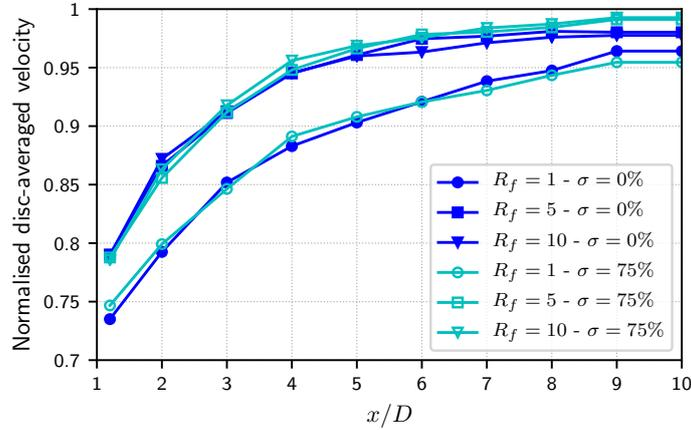
**FIGURE 5.6:** Comparison of the numerical disc-averaged velocities obtained for three filling ratios  $R_f$  and two standard deviations  $\sigma(\lambda)$  ( $TSR=3.67$ ,  $\lambda = 4.5$  m,  $I_\infty=15\%$ ).
