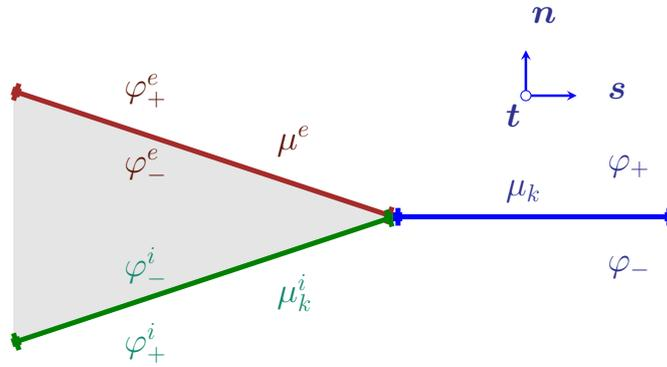
**FIGURE 2.4:** Schematic representation of a thick blade trailing edge : side view of the extrados and intrados faces along the trailing edge, and the dummy face following the trailing edge at the onset of the wake.
