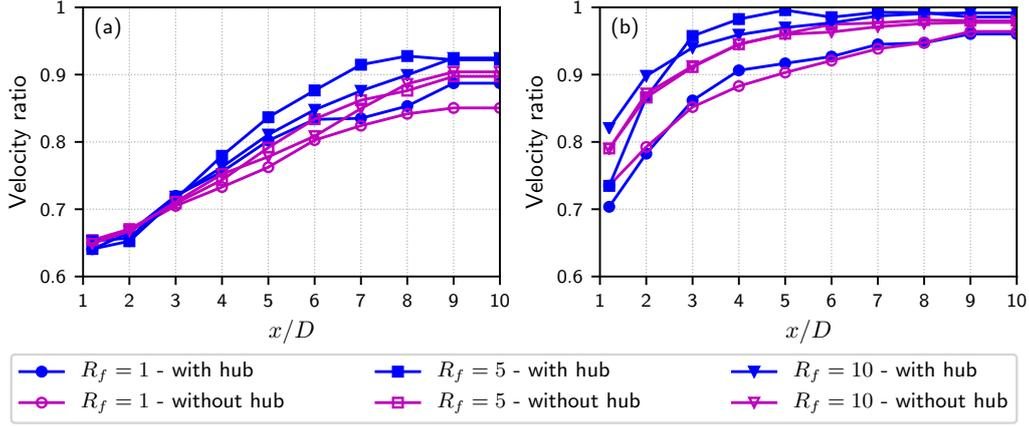
**FIGURE 5.5:** Comparison of the numerical disc-averaged velocities obtained for three filling ratios  $R_f$  and two turbulence intensities ( $TSR=3.67$ ,  $\lambda = 4.5$  m,  $\sigma = 0\%$ ). (a)  $I_\infty=1.5\%$ . (b)  $I_\infty=15\%$ .
