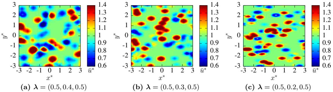
**FIGURE 3.6:** Example of velocity field provided by the ambient turbulence model for  $I_\infty = 15\%$ ,  $N = 1000$  structures and different structure sizes ( $R_f = 1.9, 1.5$  and  $1.0$  respectively). Slice at  $z = 0$  of the 3D reconstructed velocity field of size  $6 \times 6 \times 6$ .
