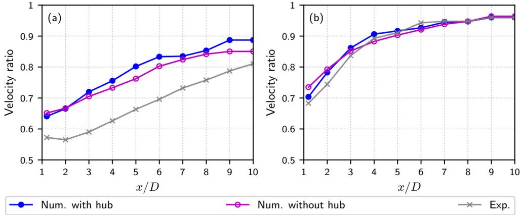
**FIGURE 5.4:** Comparison of the experimental and numerical disc-averaged velocities ( $TSR=3.67$ ,  $\lambda = 4.5$  m,  $\sigma(\lambda) = 0\%$  and  $R_f=1$ ). (a)  $I_\infty=1.5\%$ . (b)  $I_\infty=15\%$ .
