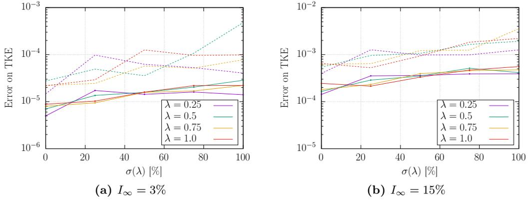
**FIGURE 3.10:** Average error (full lines) and maximal error (dashed lines) on the value of the TKE  $K$  plotted against the variance  $\sigma(\lambda)$  allowed around average turbulent structure sizes  $\lambda$ , for various size of turbulent structures  $\lambda$ . In all cases :  $I_\infty = 3\%$ ,  $R_f = 5$ , and the sub-function  $f_\lambda$  uses the Gaussian kernel.
