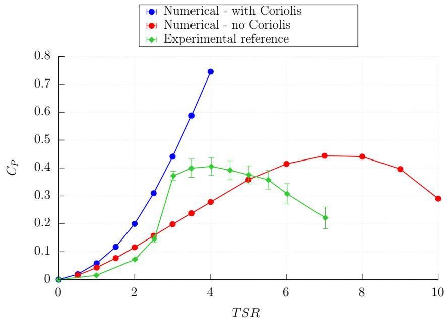
**FIGURE 1.10:** Current power curve of the IFREMER turbine computed using two different versions of the current Dorothy software power calculation, compared to flume tank experimental data provided by IFREMER.
