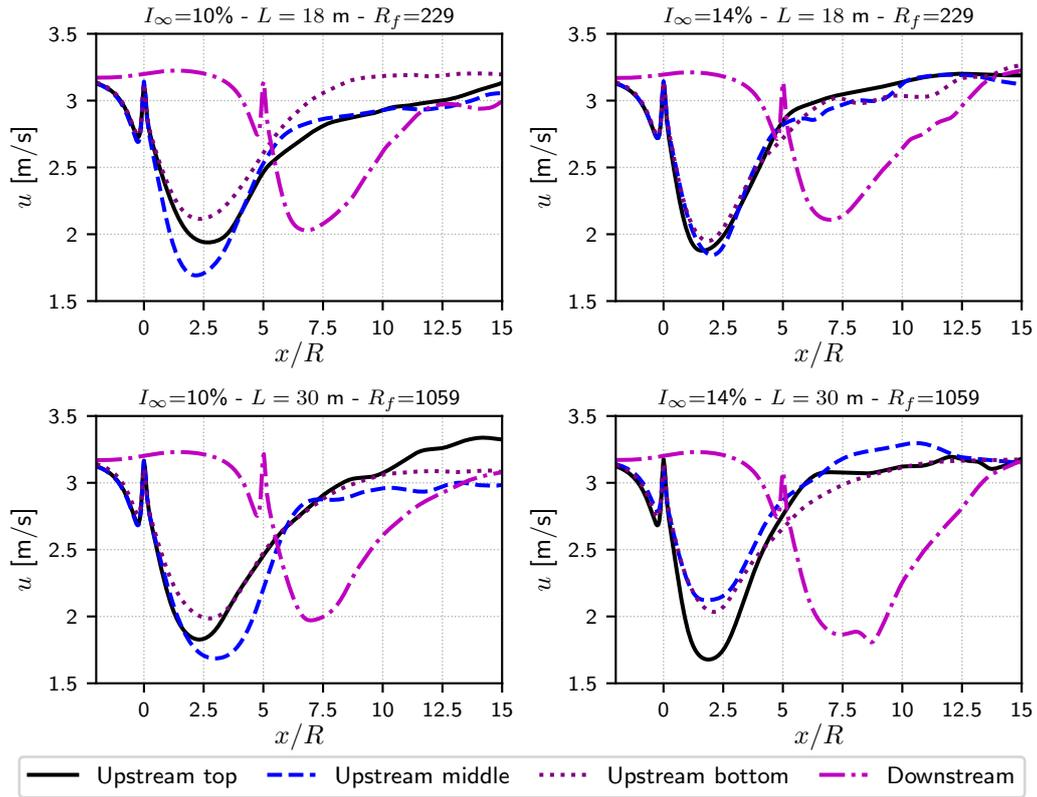
**FIGURE 5.11:** Time-averaged wake lines obtained for two turbulence intensities and two integral length scales ( $TSR=4.1$ ,  $\sigma(\lambda) = 75\%$ ). For each turbine, the corresponding line passes through its centre.
