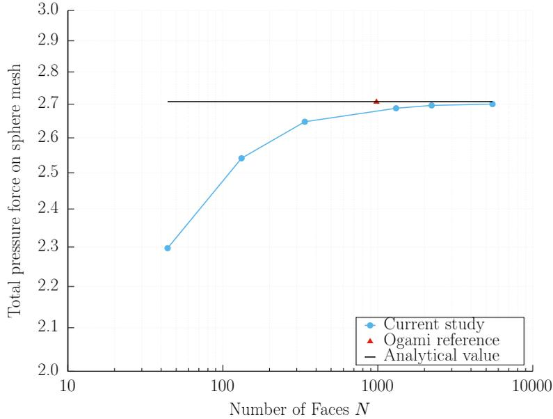
**FIGURE 2.15:** Value of the total pressure force on the accelerated sphere mesh using increasingly refined meshes, compared to the analytical value and the result obtained by Ogami.
