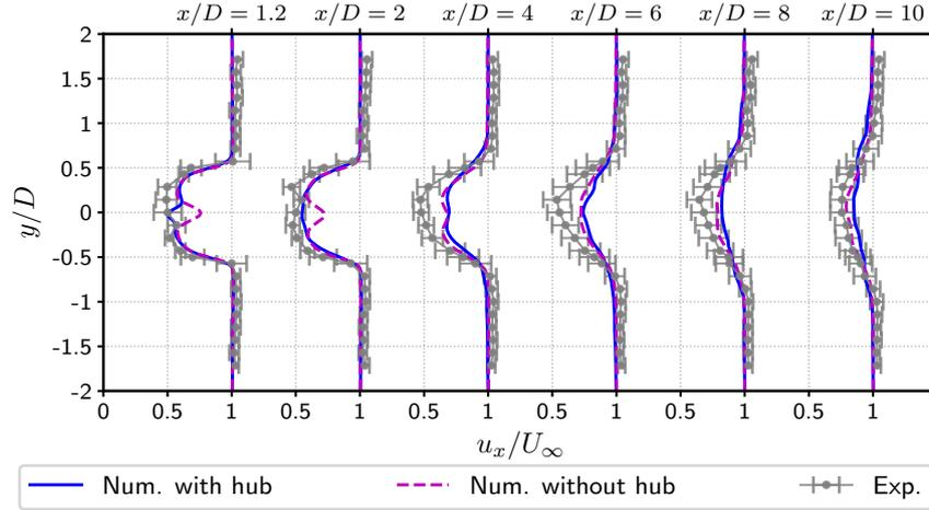
**FIGURE 5.3:** Comparison of the experimental velocity profiles with the numerical results obtained with and without nacelle, for  $I_\infty=1.5\%$ ,  $TSR=3.67$ ,  $\lambda = 4.5$  m,  $\sigma(\lambda) = 0\%$  and  $R_f=1$ .
