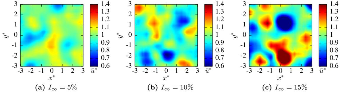
**FIGURE 3.4:** Examples of velocity fields provided by the Synthetic Eddy model for  $N = 1000$  structures of fixed size  $\lambda = 1$  ( $R_f = 19.4$ ) and different values of  $I_\infty$ . Slice at  $z = 0$  of the 3D reconstructed velocity field of size  $6 \times 6 \times 6$ .
