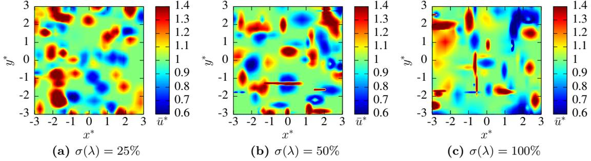
**FIGURE 3.7:** Example of velocity field provided by the ambient turbulence model for  $I_\infty = 15\%$ ,  $N = 1000$  structures of average sizes  $\lambda = 0.5$  and increasing variations allowed around this average ( $R_f = 2.4$ ). Slice at  $z = 0$  of the 3D reconstructed velocity field of size  $6 \times 6 \times 6$ .
