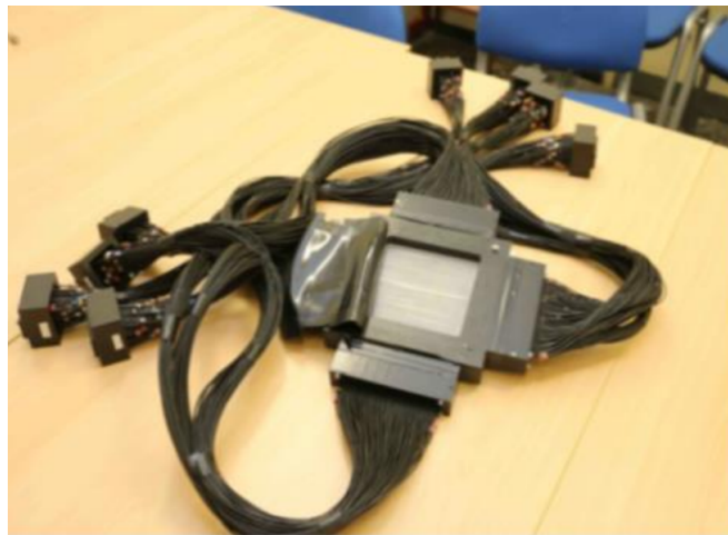
Figure 1.6: Photo of the hodoscope with scintillating fibers coupled to PMTs.
