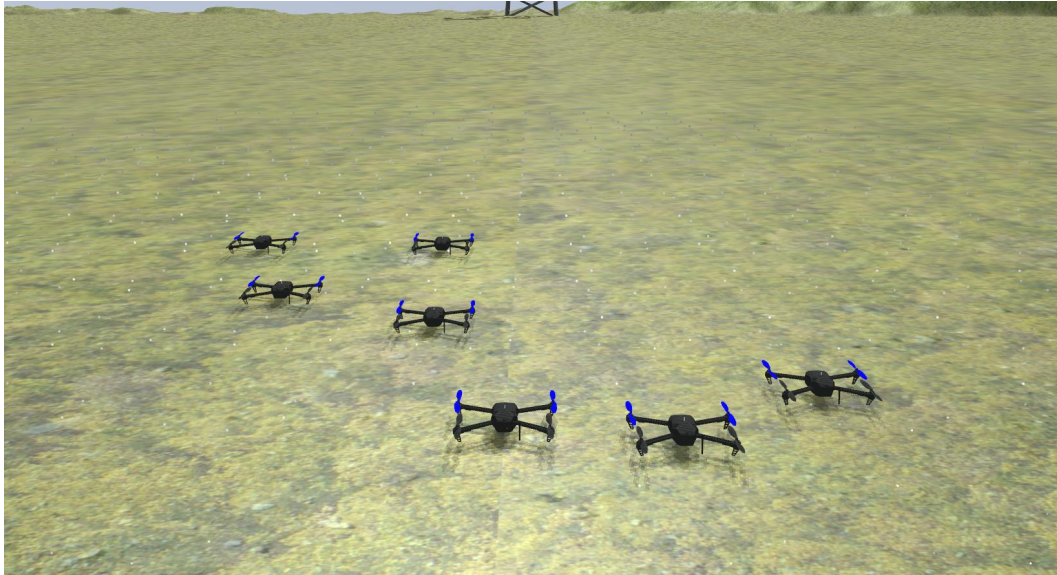
Figure 7.1.: A screenshot of the simulation environment from Gazebo simulator when spawning several quadrotors. The robots are initiated randomly in the environment.
