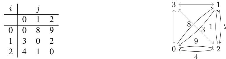
Figure 2.1: A transition table giving the transition times between the task i and j and the corresponding graph such that the initial state is the node 3 connected to each other state with gray arcs and no cost.
