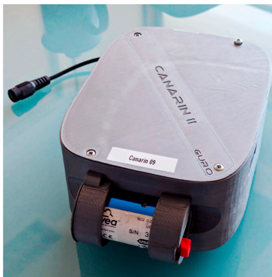
Figure 2. Canarin II in grey. The Cairnsens NO 2 is conveniently attached to it.
