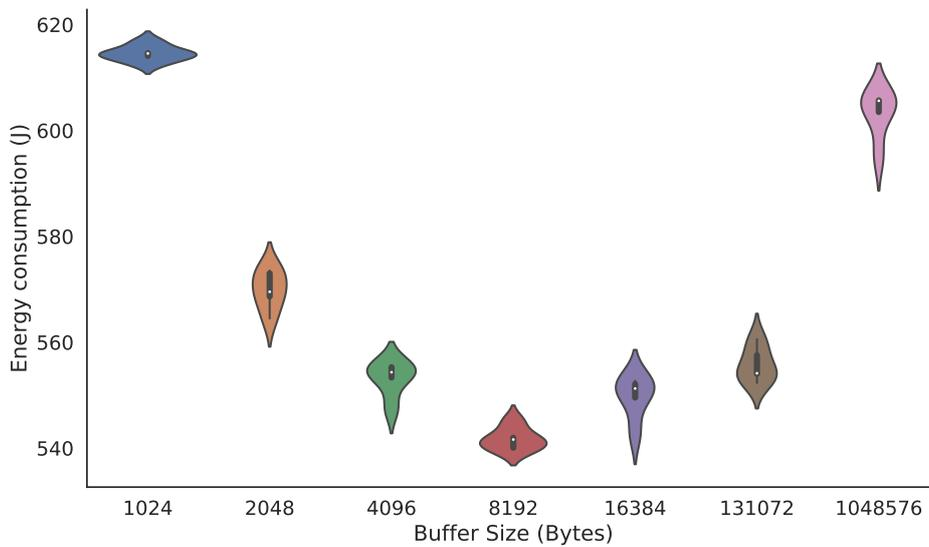
Figure 7.5: Energy consumption to read files with different buffer sizes.
