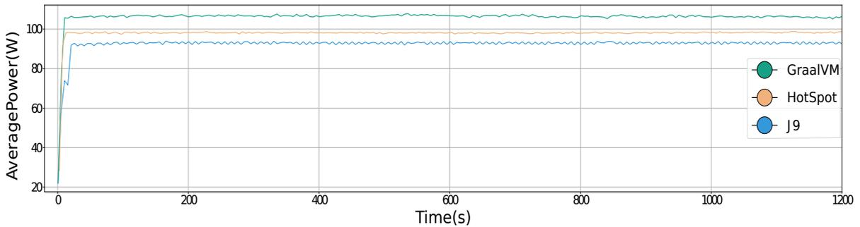
Figure 5.4: Power consumption of Scrabble-as-a-Service for HOTSPOT, GRAALVM &amp; J9.
