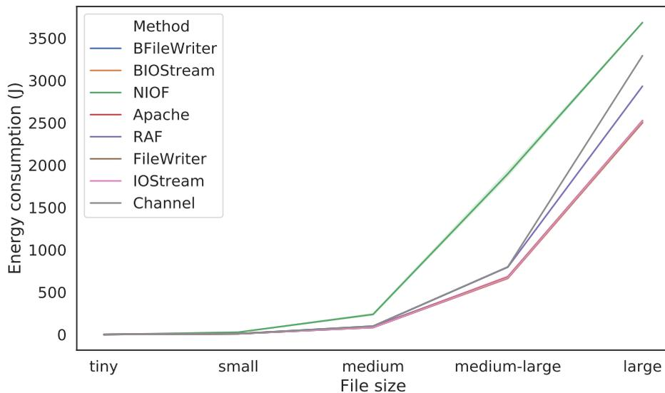
Figure 7.7: Energy consumption to write files for several file sizes.
