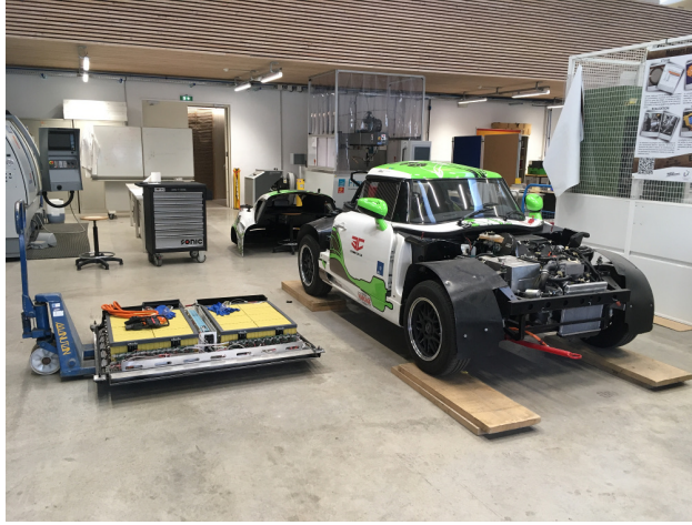
Figure 3.9: The PGO e-Hemera at IMT Mines Alès. Hood and trunk cover have been removed.
