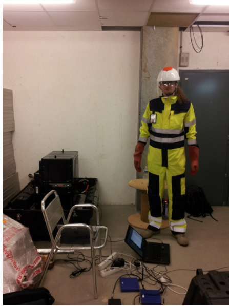
Figure 3.3: Protection equipment worn to setup the tests in the Fluence battery pack.
