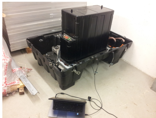
Figure 3.21: Measuring link quality inside a Fluence pack: during the test.
