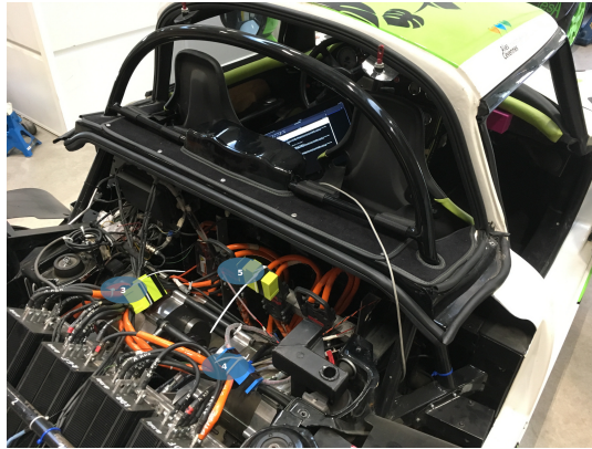
Figure 3.50: Mote placement at the back of the PGO, near the engine, for the drive test.
