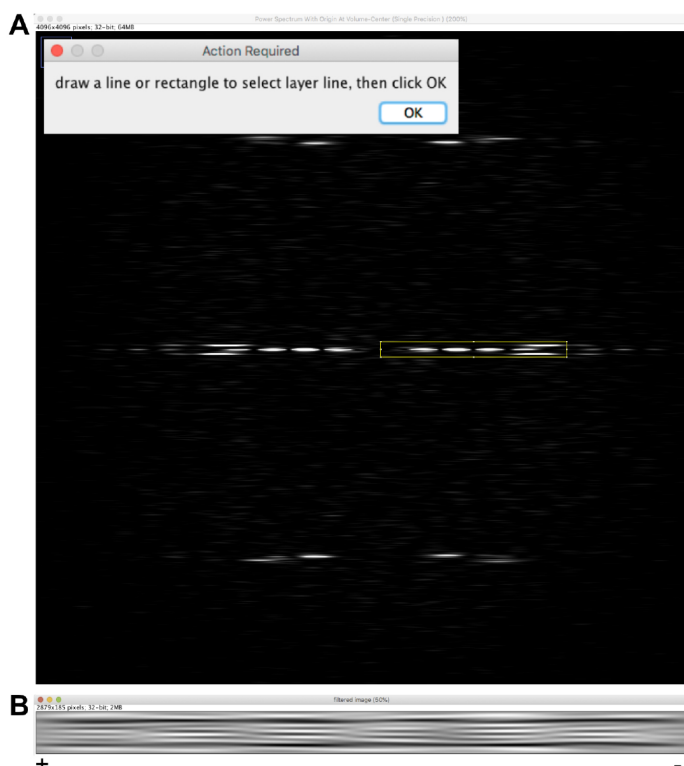
Figure 6. Microtubule image filtering. A. Selection of J_0 and of the first peak J_N . B. Filtered image. The moiré pattern displays an arrowhead shape that points toward the left of the image.
