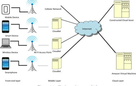
Figure 2.9: Cloulet architecture [93].
