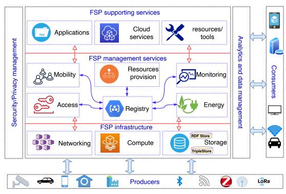
Figure 3.2: Microservices architecture for FSP
