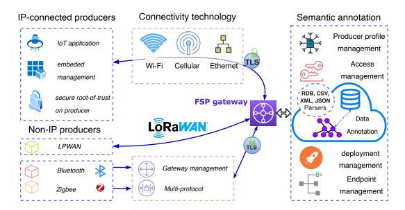
Figure 4.2: General interaction model in IoT producer layer
