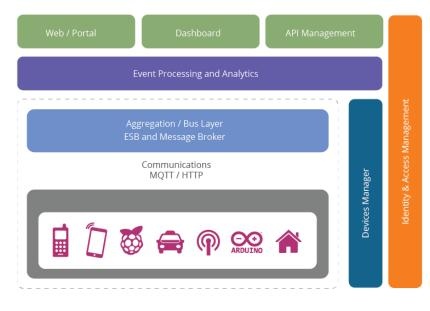
Figure 2.3: Reference architecture for IoT [48].
