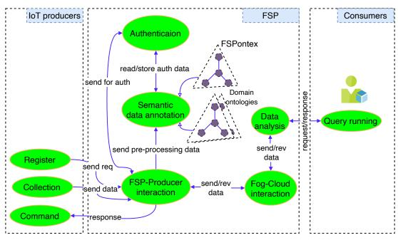
Figure 5.8: Data interaction in the FSP architecture
