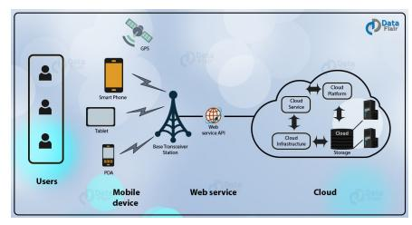
Figure 2.7: Mobile Cloud Computing architecture [84].
