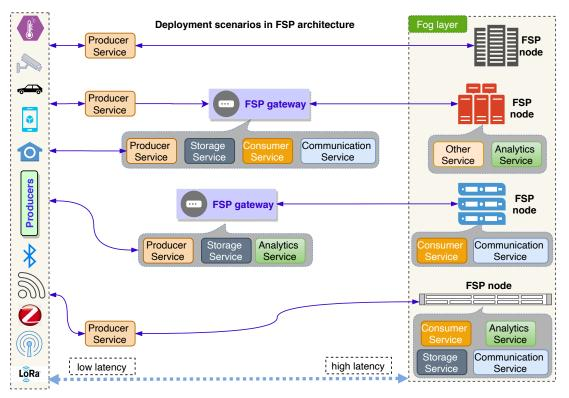
Figure 3.6: Services deployment model in FSP
