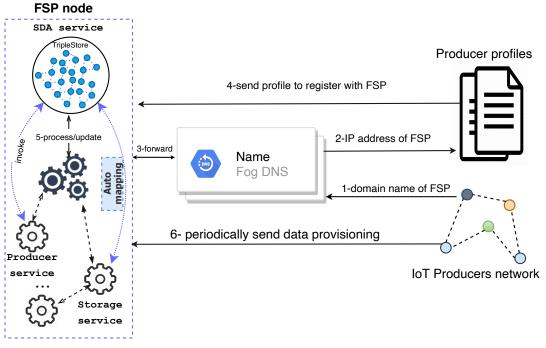
Figure 4.6: IoT producers registration service.
