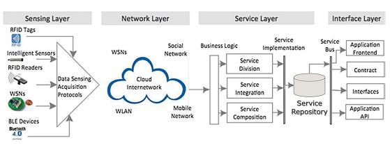
Figure 2.4: Service-oriented Architecture for IoT [54].
