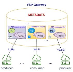
Figure 5.7: FSP gateway for network interoperability
