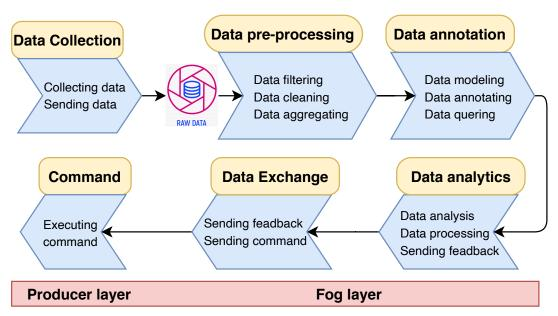
Figure 3.3: Data management in the FSP architecture
