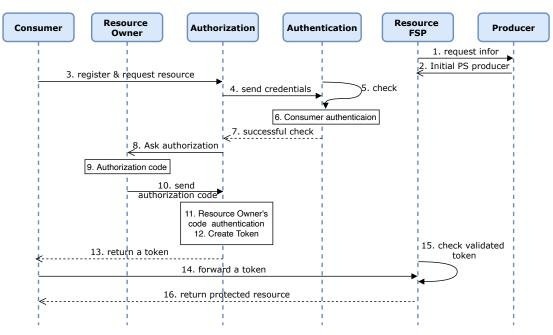
Figure 4.7: The register and access procedure for consumers.
