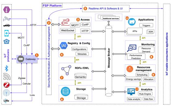
Figure 3.4: Interaction model in FSP
