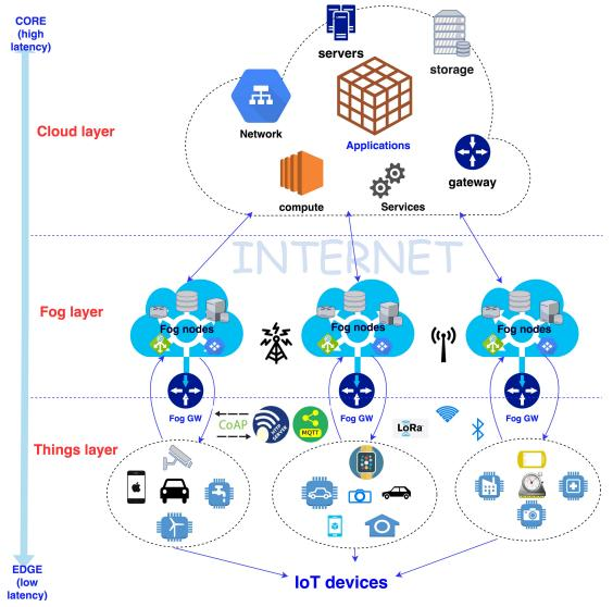
Figure 2.10: A model of Fog computing.
