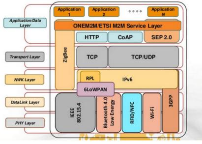
Figure 2.2: Heterogeneous IoT standard protocols.
