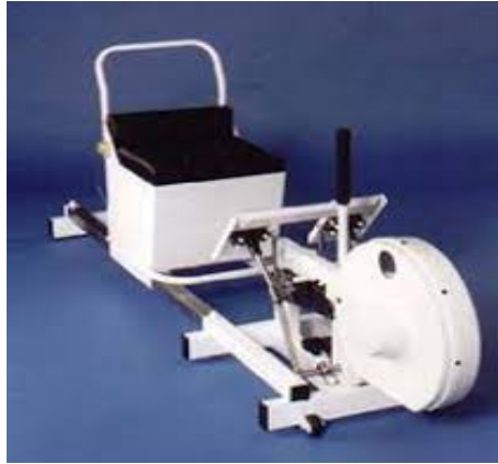
Figure 25. The Nottingham Leg Power Rig machine to evaluate the Explosive Leg Extensor Power
