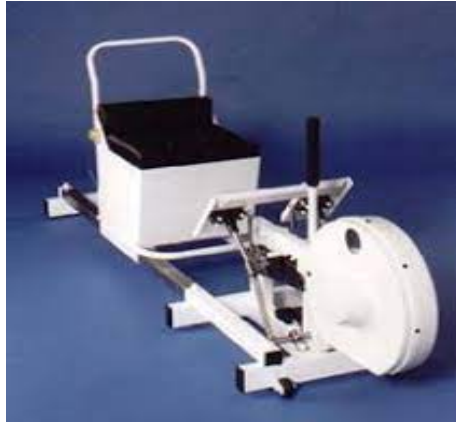
Figure 25. The Nottingham Leg Power Rig machine to evaluate the Explosive Leg Extensor Power
