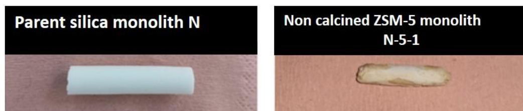
Figure S3. Photographs of parent silica monolith N and ZSM-5 nanosheets monolith N-5-1 (the length is smaller than the parent's one because a part was cut for TGA analysis)
