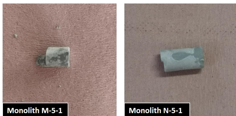
Figure 13. Photographs of the synthesized monoliths M-5-1 and N-5-1 after mercury intrusion-extrusion experiments
