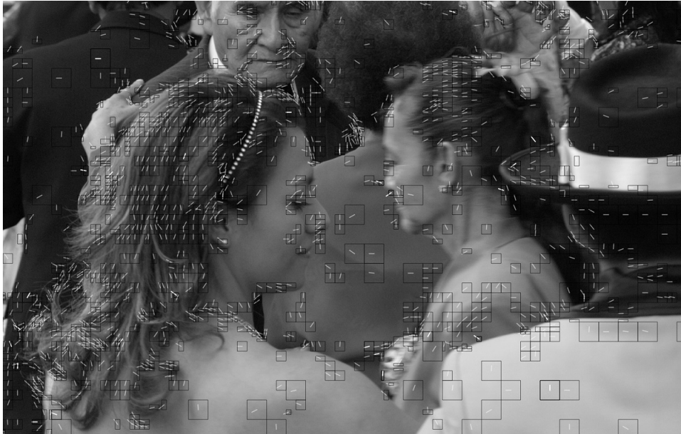
FIGURE 5.4: Correlation between content texture and implicitly derived angular IPMs using DIMD.
