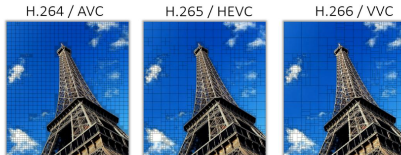
FIGURE 3.4: Comparison between partitionings of AVC, HEVC and VVC.
