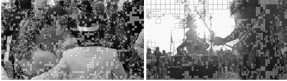
FIGURE 5.5: Spatial distribution of DIMD blocks in different sequences of Tango ( 3840 \times 2160 ) and RitualDance ( 1920 \times 1080 ).
