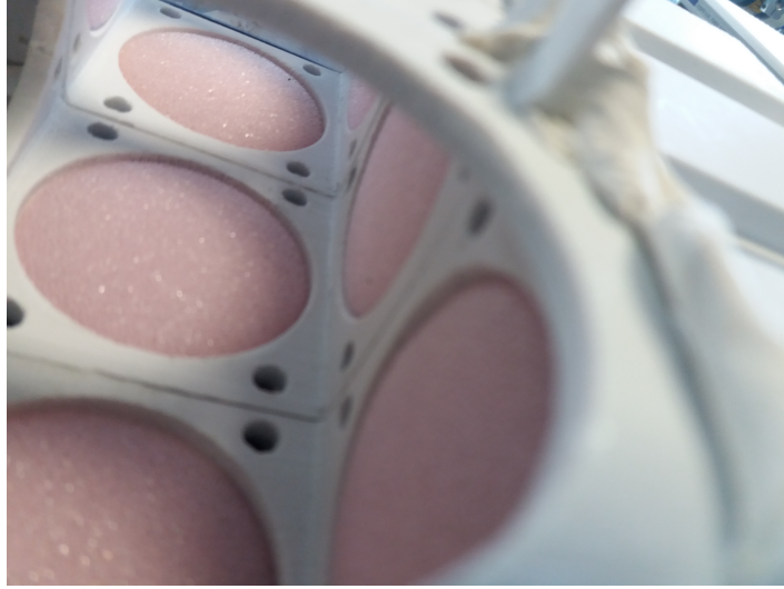
Figure 3.54: View of the waveguide interior. In pink, the layers of foam applied in front of the loudspeakers without interfering with the mechanical vibration of the diaphragms, and maintaining the “flush” condition of the liner.
