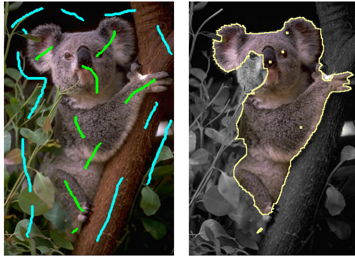
Figure 9.8: Foreground (green) and background (blue) seeds are shown in the left and the resulting graph cut segmentation in the right.
