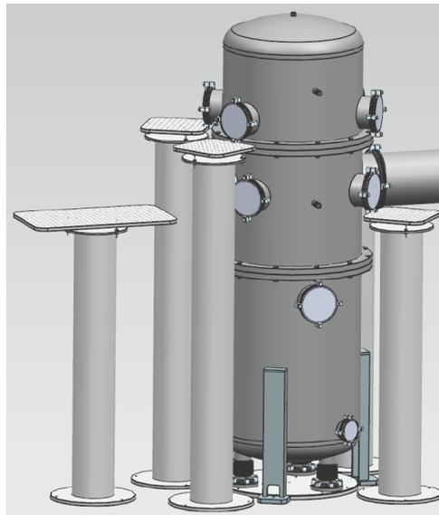
**Figure 7.6:** CAD drawing of the Filter Cavity mirrors suspension and picture of the micro-tower hosting them. Credit : A. Bertolini
