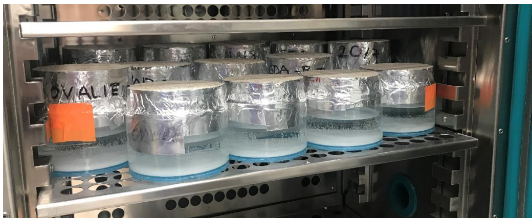
Figure 2.7 - Essai coupelle humide.
