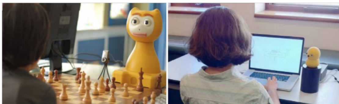
Figure 3.5: Examples of social robots for learning. (i) iCat robot teaching young children to play chess Pereira et al. (2008) (Left) and (ii) Keepon robot tutoring an adult in a puzzle game Leyzberg et al. (2014) (Right)
