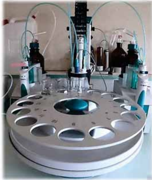
Fig. 5. Titrator used to measure the chloride content
