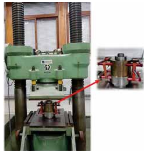
Fig. 2. Sintco press and an extraction mold to extract interstitial solution from concrete
