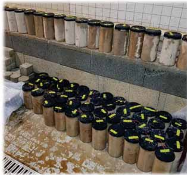
Fig. 5. Cathodes in wet curing room after casting before demolding
