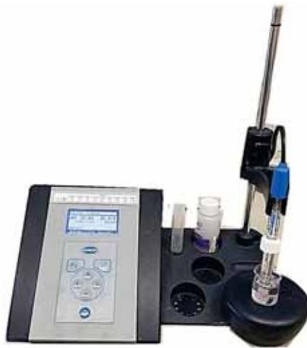
Fig. 3. pH meter with a combined pH electrode.
