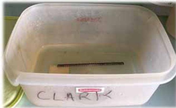
Fig. 2. Reinforcement bar soaked in a Clark solution
