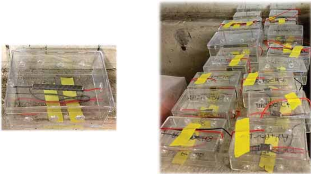
Fig. 7. Reinforcement bars placed in humidity room (photograph taken directly after placing the rebars in the room)
