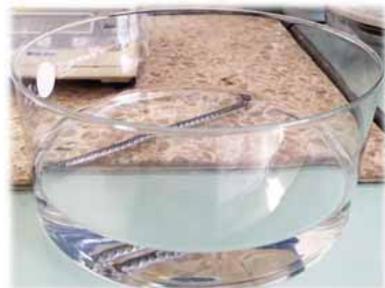
Fig. 4. Rebar totally immersed in acetone
