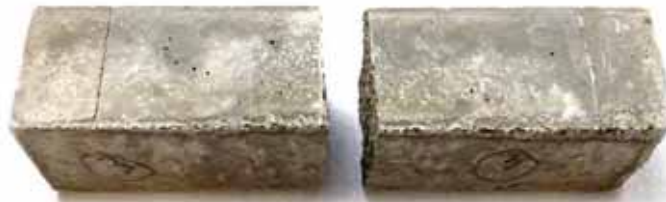
Fig. 9. Two half-prisms obtained from bending test
