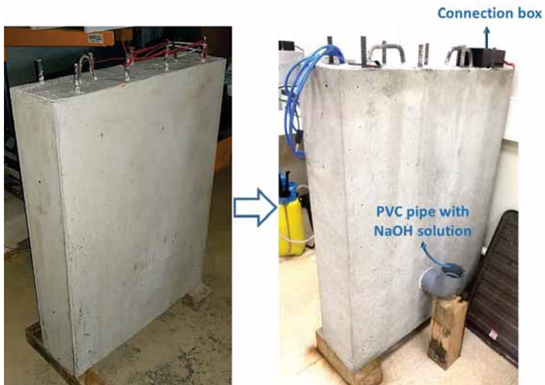
Fig. 14. Wall after demolding and installation of PVC tube
