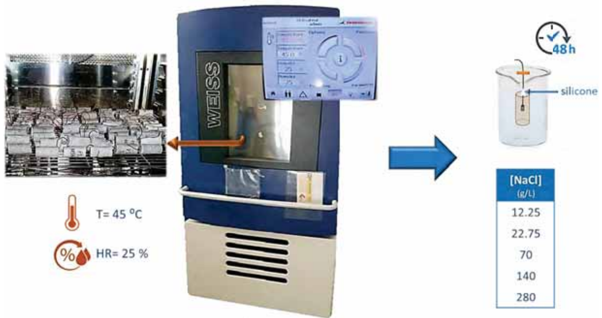
Fig. 10. Preconditioning of anode samples (drying then soaking in NaCl saline solution)
