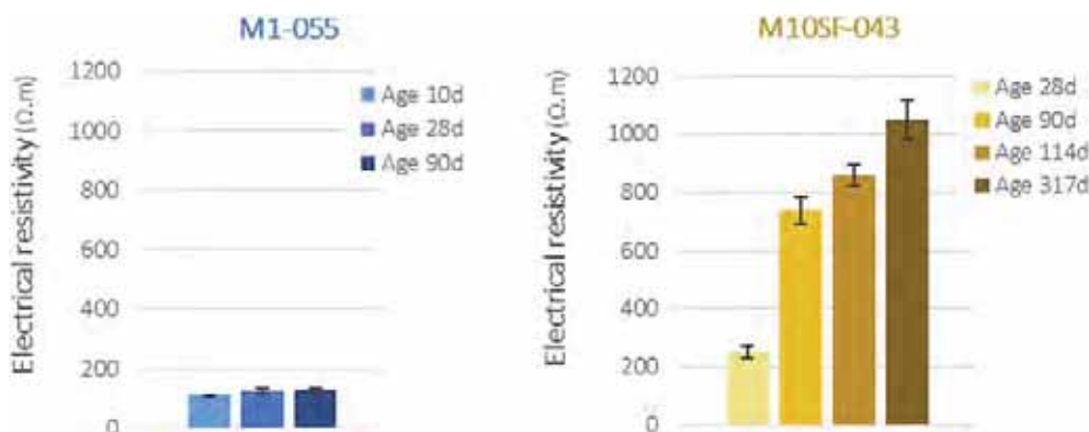
Fig. 1. Monitoring of electrical resistivity of M1-055 and M10SF0-43 according to RILEM TC-154 EMC.
