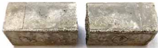
Fig. 9. Two half-prisms obtained from bending test
