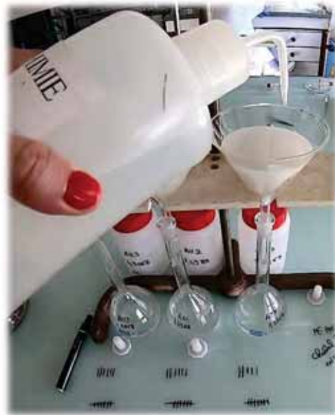
Fig. 4. Description of the methodology used to prepare solutions for measuring the total chloride contents
