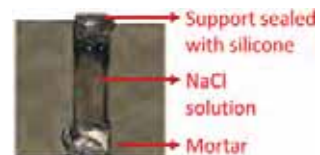
Fig. 3. Top view at anode level after addition of the saline solution.
