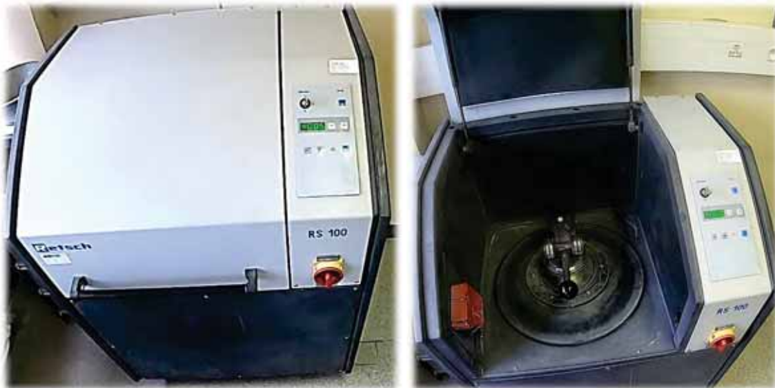
Fig. 3. Grinding machine used to transform mortar/concrete samples into fine powder
