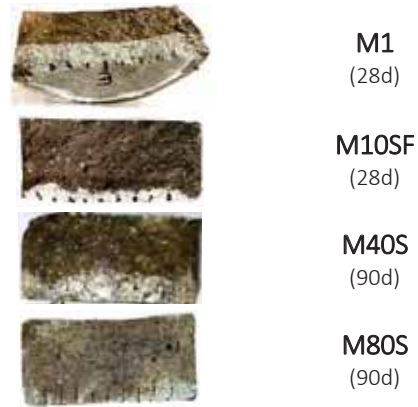
Fig. 7. Examples of chloride penetration fronts of mortar formulations
