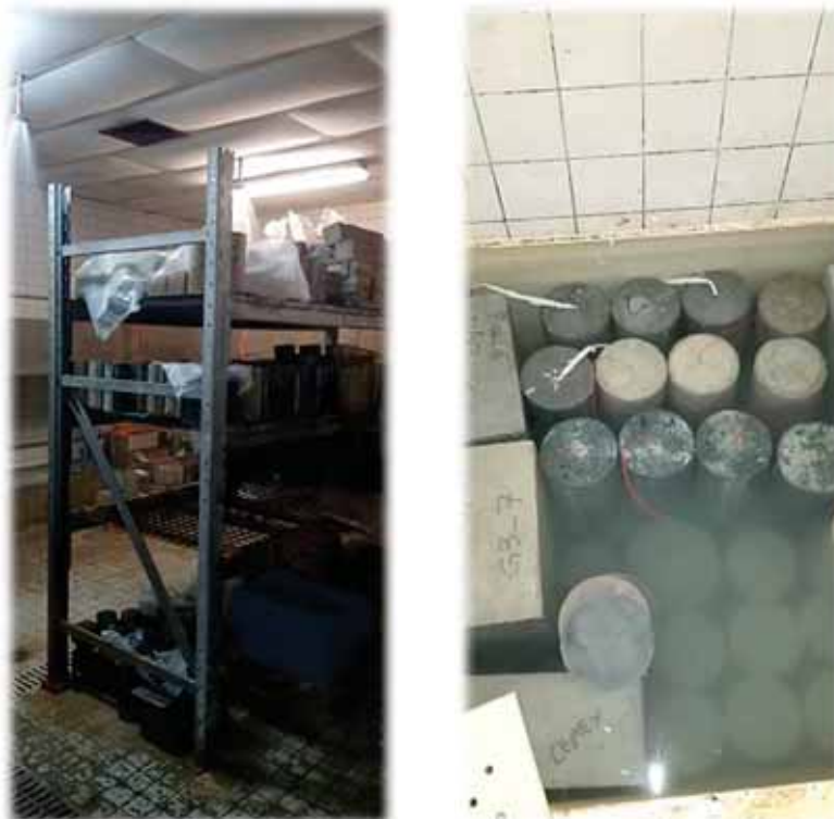
Fig. 6. Wet curing of cathodes (on the left) and water immersion of cathodes samples (on the right)
