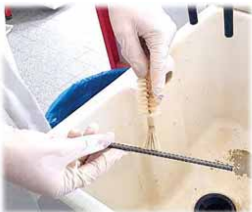
Fig. 3. Rinsing with water and brushing steel after cleaning with Clark solution
