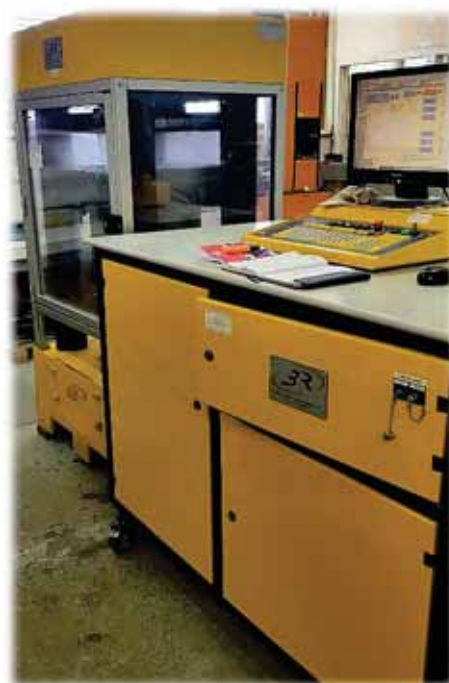
Fig. 8. Concrete press machine
