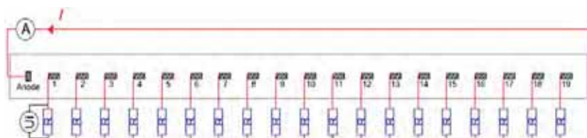
Fig. 7. Connections of the acquisition system when all cathodes are connected to the anode.
