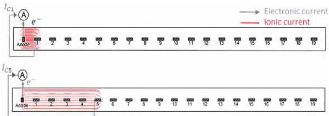
Fig. 12. Streamlines of the currents exchanged between the anode and each of the cathodes C_1 and C_5 .
