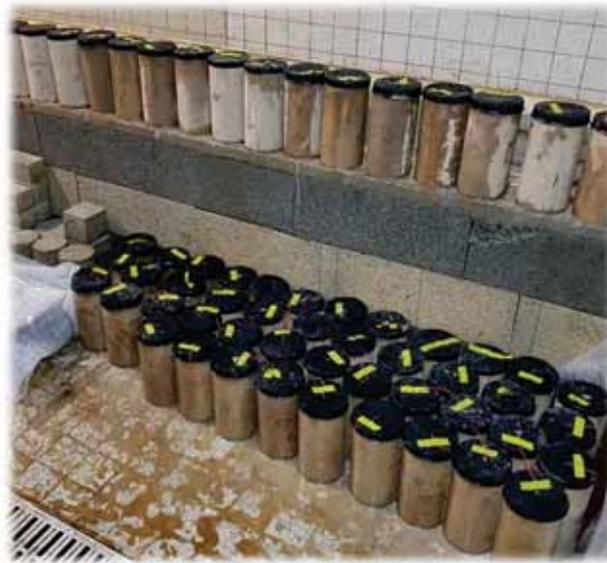
Fig. 5. Cathodes in wet curing room after casting before demolding
