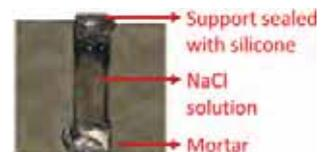
Fig. 3. Top view at anode level after addition of the saline solution.
