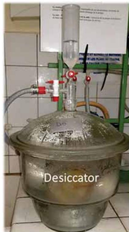
Fig. 2. Saturation device
