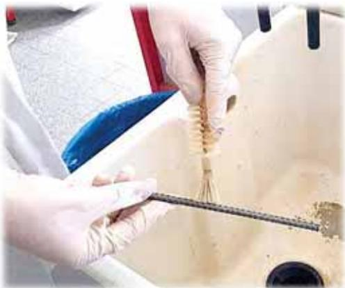
*Fig. 3. Rinsing with water and brushing steel after cleaning with Clark solution*
