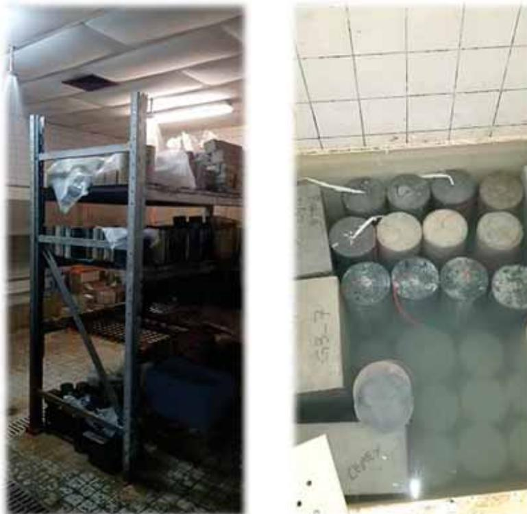
Fig. 6. Wet curing of cathodes (on the left) and water immersion of cathodes samples (on the right)
