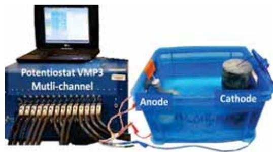
Fig. 1. Experimental set-up of the anode-cathode connection
