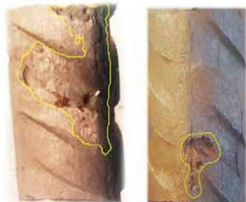
**FIGURE 6** Examples of microscopic inspections on the anode steel bars showing the localized corroded areas [Color figure can be viewed at [wileyonlinelibrary.com](http://wileyonlinelibrary.com)]
