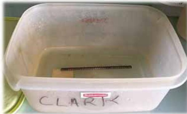
*Fig. 2. Reinforcement bar soaked in a Clark solution*
