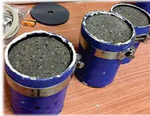
Fig. 3. Samples fixed in rubber sleeves
