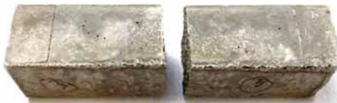
Fig. 9. Two half-prisms obtained from bending test
