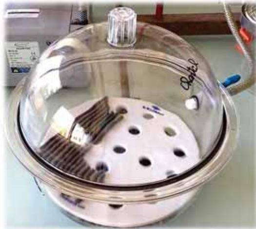
Fig. 5. Desiccator containing cleaned steels
