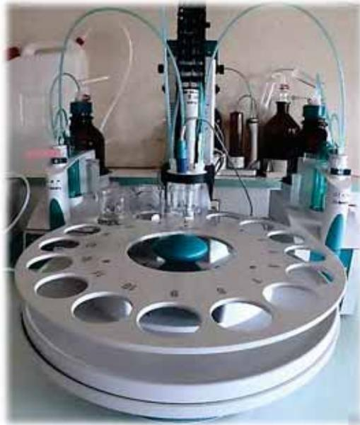
Fig. 5. Titrator used to measure the chloride content
