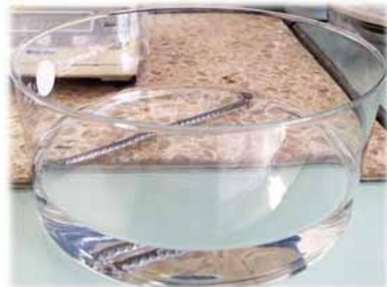
*Fig. 4. Rebar totally immersed in acetone*
