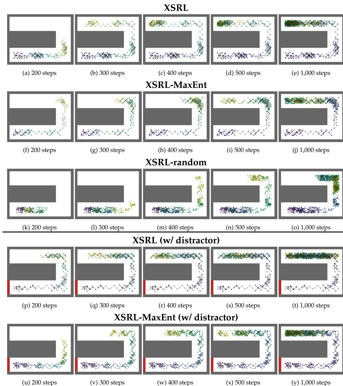
Figure 12. Visualization of the TurtleBot Maze exploration, where the color spectrum of the robot's position goes from purple (start of the episode) to yellow (end of the episode). The results obtained in the regular TurtleBot Maze environment correspond to: (a)-(e) XSRL, (f)-(j) XSRL-MaxEnt, (k)-(o) XSRL-random. The results obtained in TurtleBot Maze with a randomly sampled wall color correspond to: (p)-(t) XSRL, (u)-(y) XSRL-MaxEnt.
