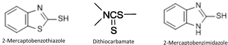
Fig. II. 22 Chemical structures of the sulfur type anti-oxidation agent.
