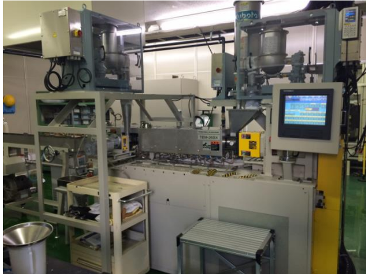
Fig. II. 7 Appearance of used twin screw extruder (JTEKT, Japan).
