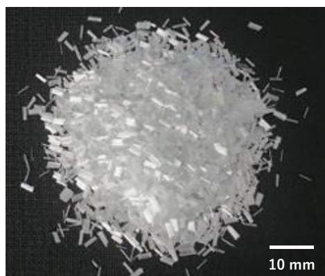
Fig. II. 3 Appearance of used GF chopped strands observed with optical microscope.
