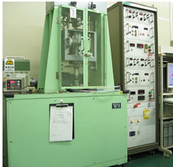
Fig. II. 39 Appearance of used tribometer in JTEKT.
