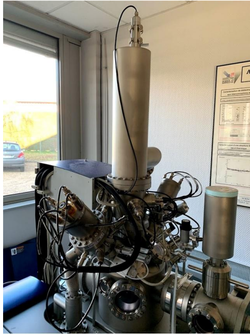
Fig. II. 42 Appearance of used ToF-SIMS.
