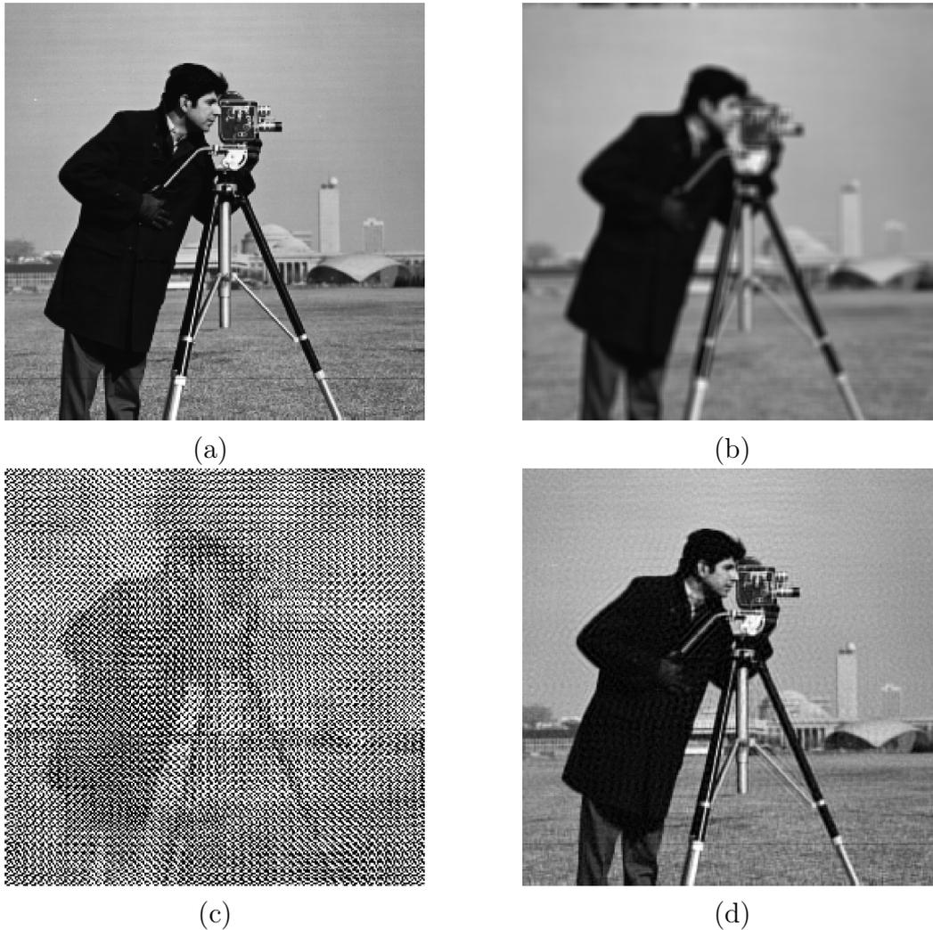
Figure 2.2: Ill conditioned inverse filter. (a): original 2D image of *cameraman* from the Matlab Image processing Toolbox. (b): output image degraded by a 2D square convolution kernel, and corrupted with an additive white Gaussian noise, (c): solution with an inverse filter, (d): regularized least square solution, with an  $l_2$  regularization
