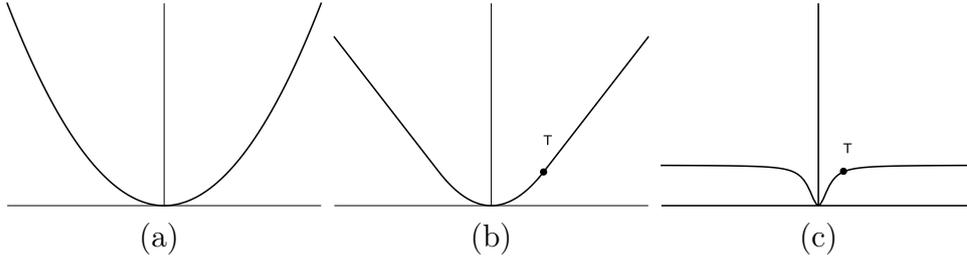
Figure 2.3: Different potential functions: (a) quadratic potential function (b) convex  $l_2l_1$  huber potential function, (c) non convex  $l_2l_0$  Geman and McClure function. The parameter  $T$  in (b) and (c) refers to the threshold. Below this threshold, the functions have a quadratic behaviour, and above it is linear or constant.
