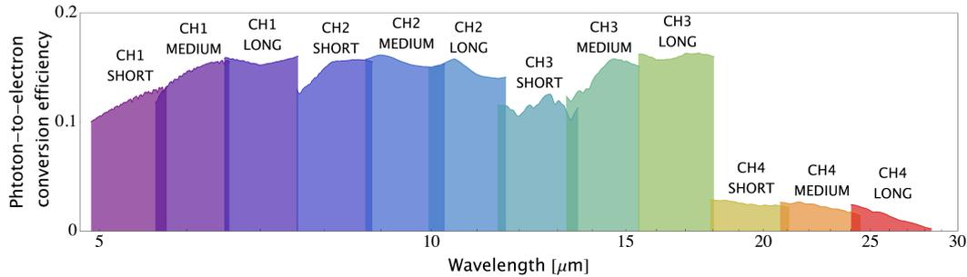
Figure 3.6: wavelength bands response for the MRS instrument.
