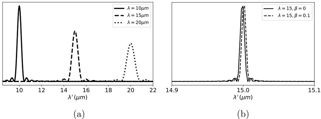
Figure 3.9: Cuts across monochromatic punctual sources, diffracted and projected onto a detector array, (a) for three monochromatic point sources at  $\lambda = 10, 15,$  and  $20 \mu\text{m}$  entering the input slit with the same spatial position  $\beta$ , and (b) for two identical punctual monochromatic sources at  $\lambda = 15 \mu\text{m}$ , but placed at different  $\beta$  (in arcseconds).
