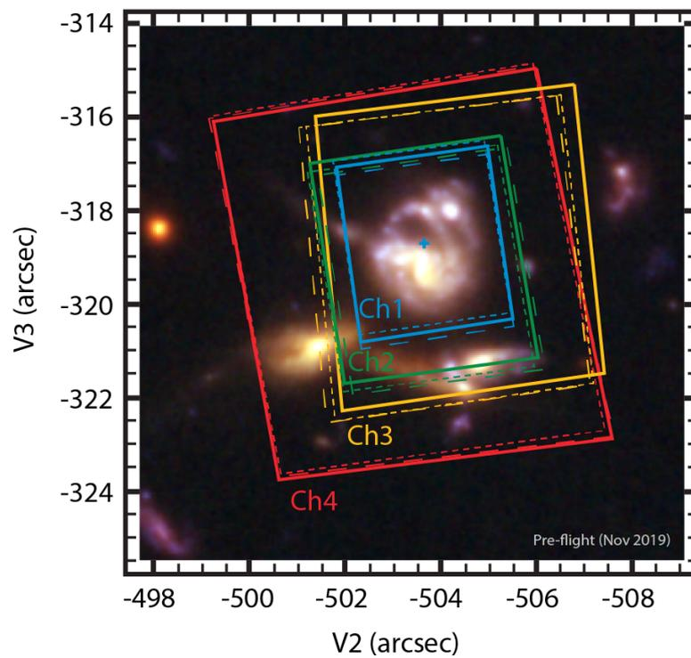
Figure 3.5: Figure showing the co-aligned spatial FOV of the four MRS spectral channels. Edited from: <https://jwst-docs.stsci.edu/mid-infrared-instrument/miri-instrumentation/miri-mrs-field-and-coordinates>
