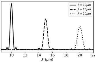
Fig. 1. The spatial position ( $\lambda' = l' T_l$ ) of the response on the detector depends on the input wavelength ( $\lambda = l T_l$ )
