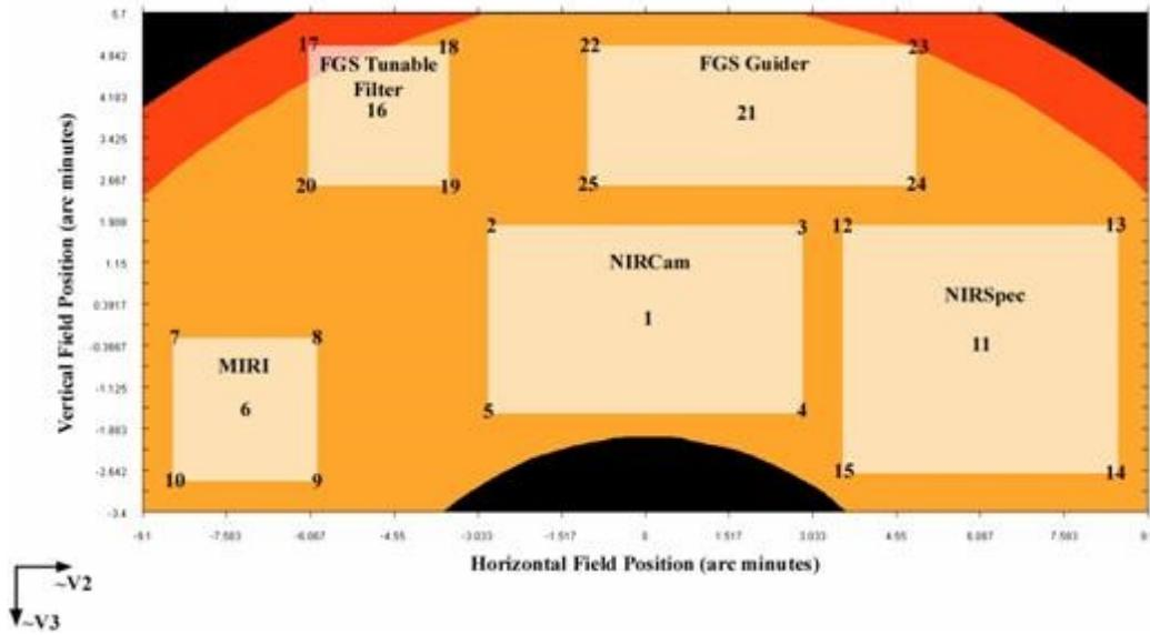
Figure 3.2: The JWST focal plane layout (<https://www.cosmos.esa.int/web/jwst-nirspec/home-old>)
