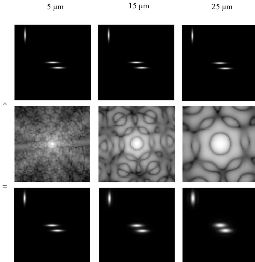
Figure 4.1: Illustration of the spatial filtering: (Top) Three monochromatic synthetic images at wavelength 5, 15 and 25  $\mu\text{m}$ . (Middle) Three monochromatic PSFs simulated with the WebbPSF simulator at the same wavelengths. (Bottom) Filtered images.
