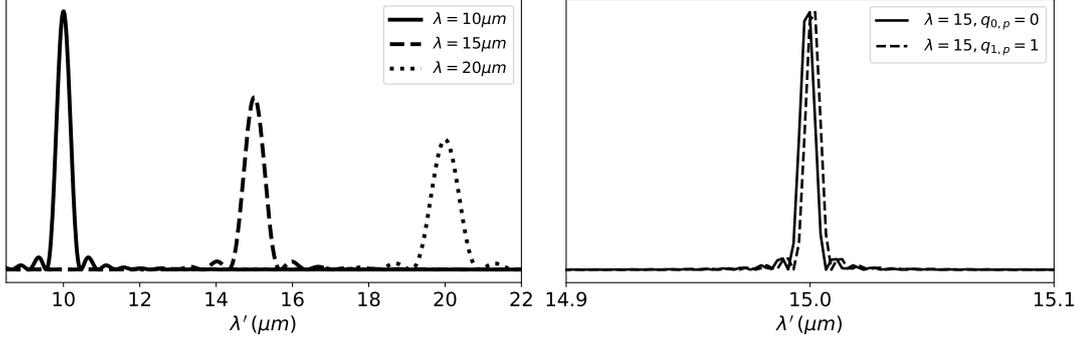
Figure 4.3: (Left) Spectral dependence of the grating response, (Right) influence of the spatial position  $j$  of the input source,  $q_{j,p}$  for a particular pointing  $p$ , on the position of the diffracted light.
