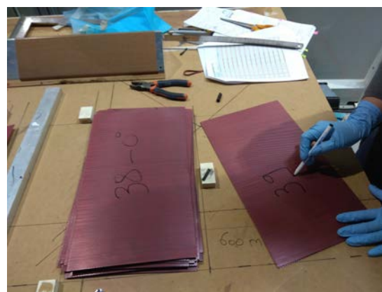
Fig. 8.2. Front and back side numbering of cut prepreg plies.
