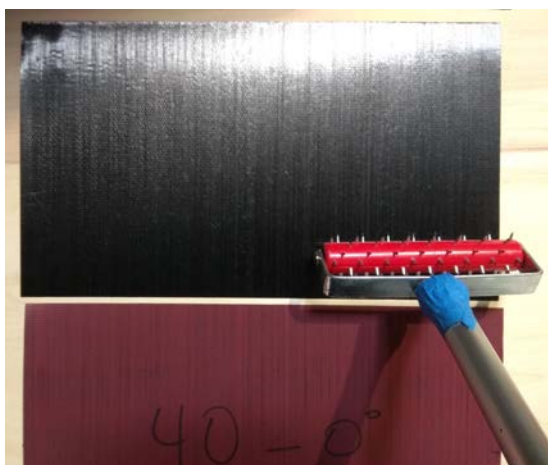
Fig. 8.3. Spyking of each ply before hand lay-up.
