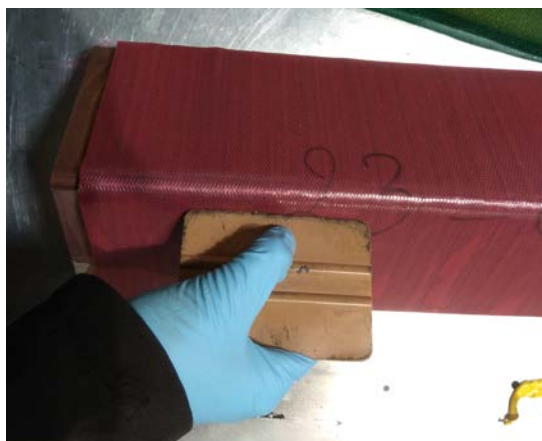
Fig. 8.4. Use of a spatula on the sides and the the thumbs at the corner of the panel to ensure good adhesion between the plies.
