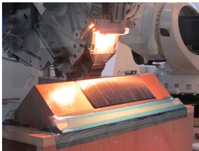
Fig. 7.2. Manufacturing of AFP L-beam panel. Lay-up time 1h05min.
