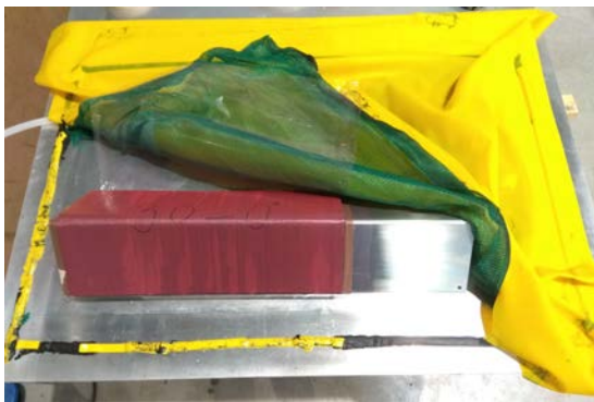
Fig. 8.5. Intermediate debulking every 3 plies during 20 min. Total lay-up time 9 h20 min.
