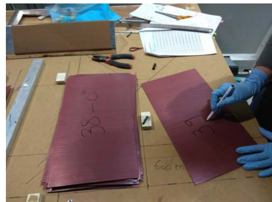
Fig. 8.2. Front and back side numbering of cut prepreg plies.
