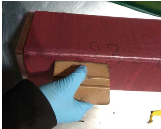
Fig. 8.4. Use of a spatula on the sides and the thumbs at the corner of the panel to ensure good adhesion between the plies.
