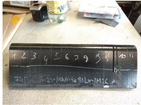
Fig. 8.8. L-beam panel after autoclave curing and mitre saw cutting.
