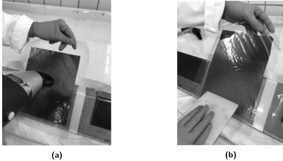
Fig. 5.7. Hand lay-up in Zumaquero et al. [2018]. (a) application of the heating of each ply using a technical hair dryer. (b) pressure smoothing of each ply using a spatula.
