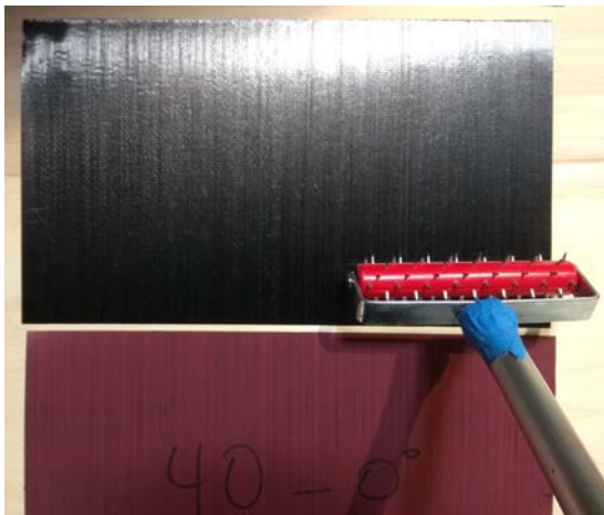
Fig. 8.3. Spyking of each ply before hand lay-up.
