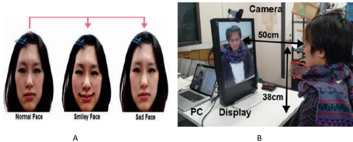
FIGURE 2.4 (A) : The facial expressions deformations Smile face and Sad face .(B) : Experiment protocol for the facial deformation in real-time [138]. This study proves that user's emotional state is influenced by the feedback of deformed facial expressions
