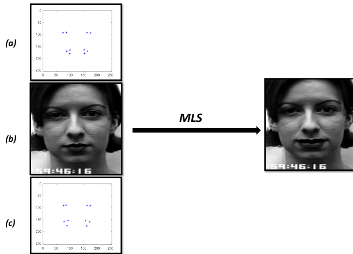
FIGURE 3.9 The MLS inputs are : (a) the detected landmarks X_c^i . (b) the detected face and (c) the target smiling landmarks determined by the model X_{c,s}^i .
