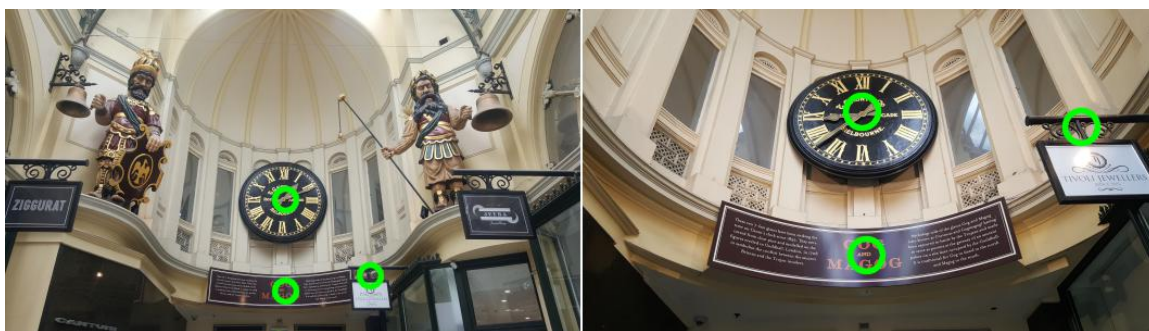
Figure 2.4: Keypoints are pixels that are easily matchable across images. In this example, the center of the green circles are keypoints matched across two viewpoints.
