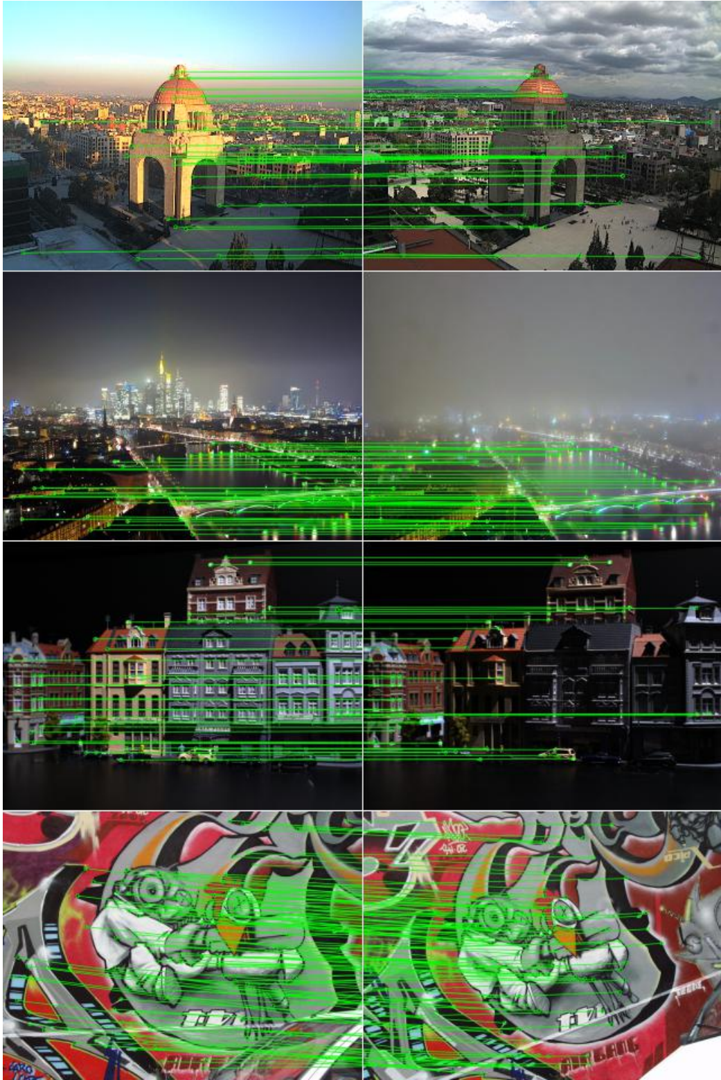
Figure 5.13: Green lines are ELF's putative matches of the proxy-descriptor before RANSAC-based homography estimation.
