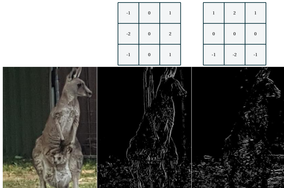
Figure 2.7: Left-Right: Image, Vertical Sobel filter, Horizontal Sobel filter. The filters compute the first order derivative of the pixel intensity along the y and x axis. It highlight the edges, i.e. , an area where the pixel intensity varies.
