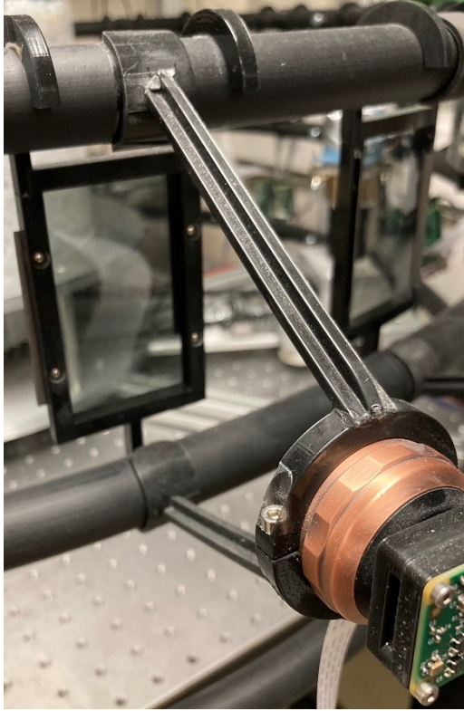
(a) Analyzing polarizers are now held by a frame, in front of each camera.
