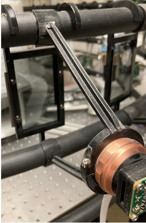
(a) Analyzing polarizers are now held by a frame, in front of each camera.
