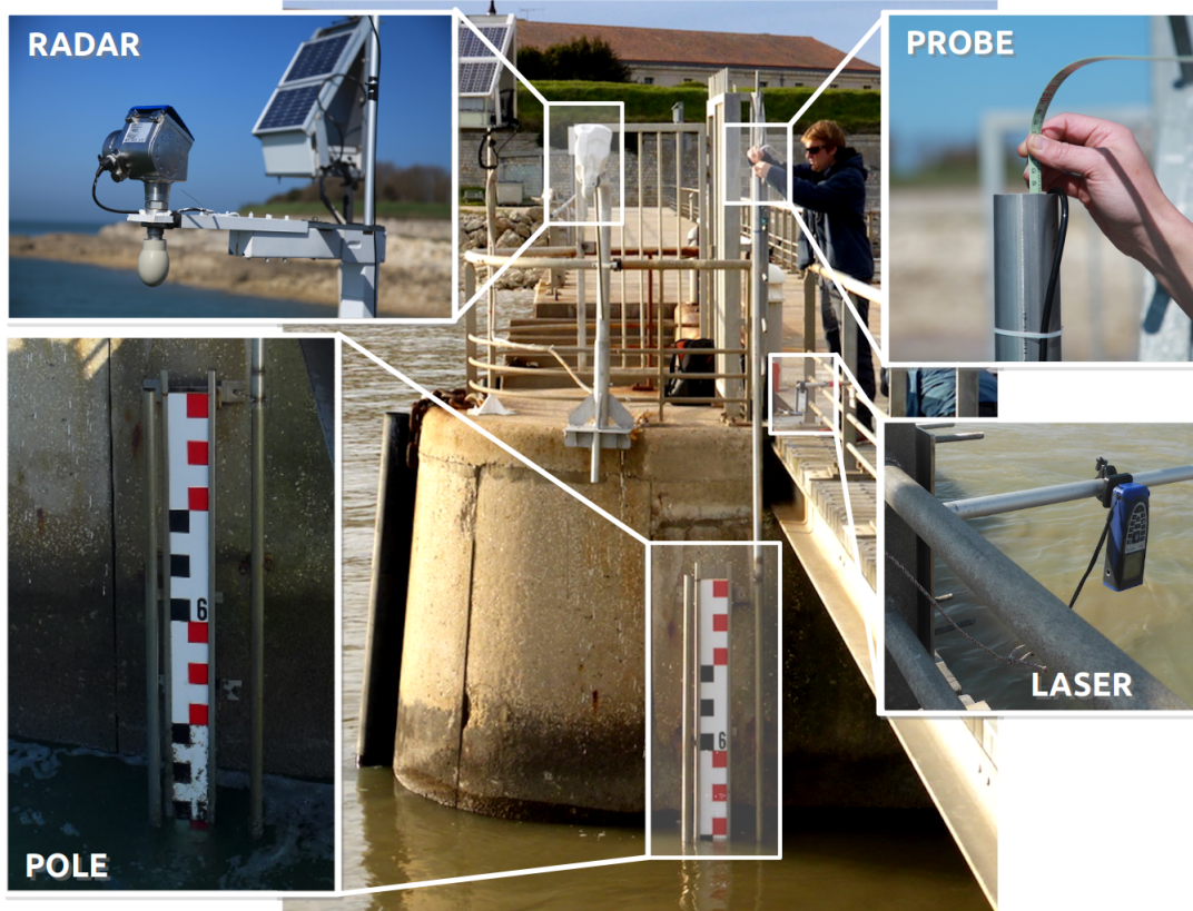
FIGURE 7.1: The four ground-based tide gauges: RADAR, POLE, PROBE and LASER.
