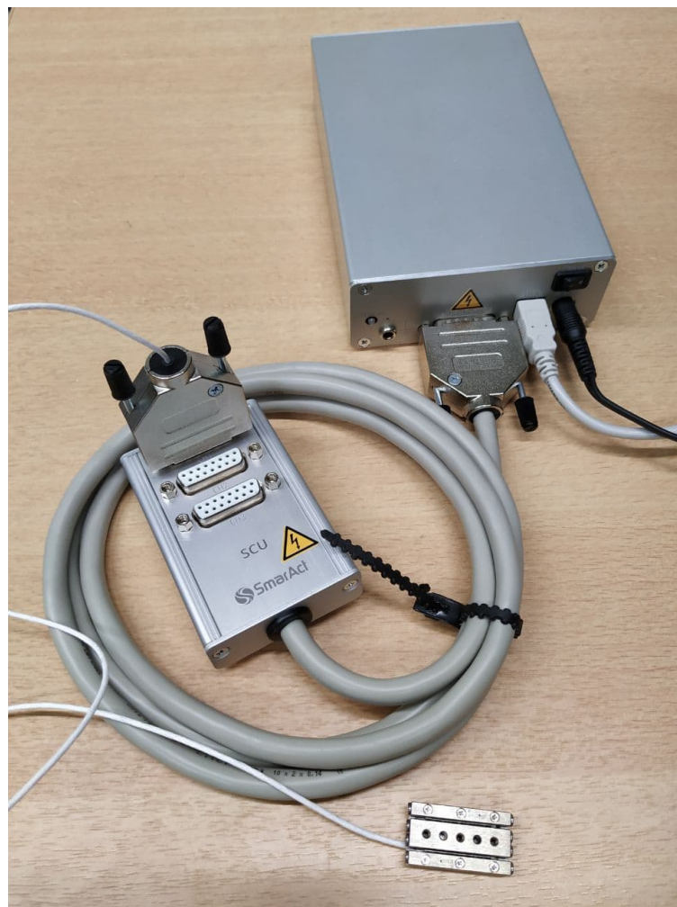
FIGURE 4.37: Connection of the controller unit and the actuator.
