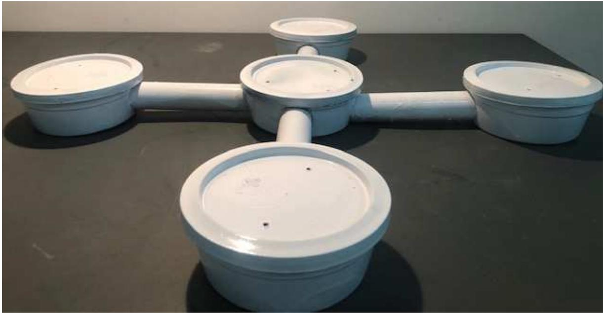
**Figure 1.** Four arms olfactometer used in this study.
