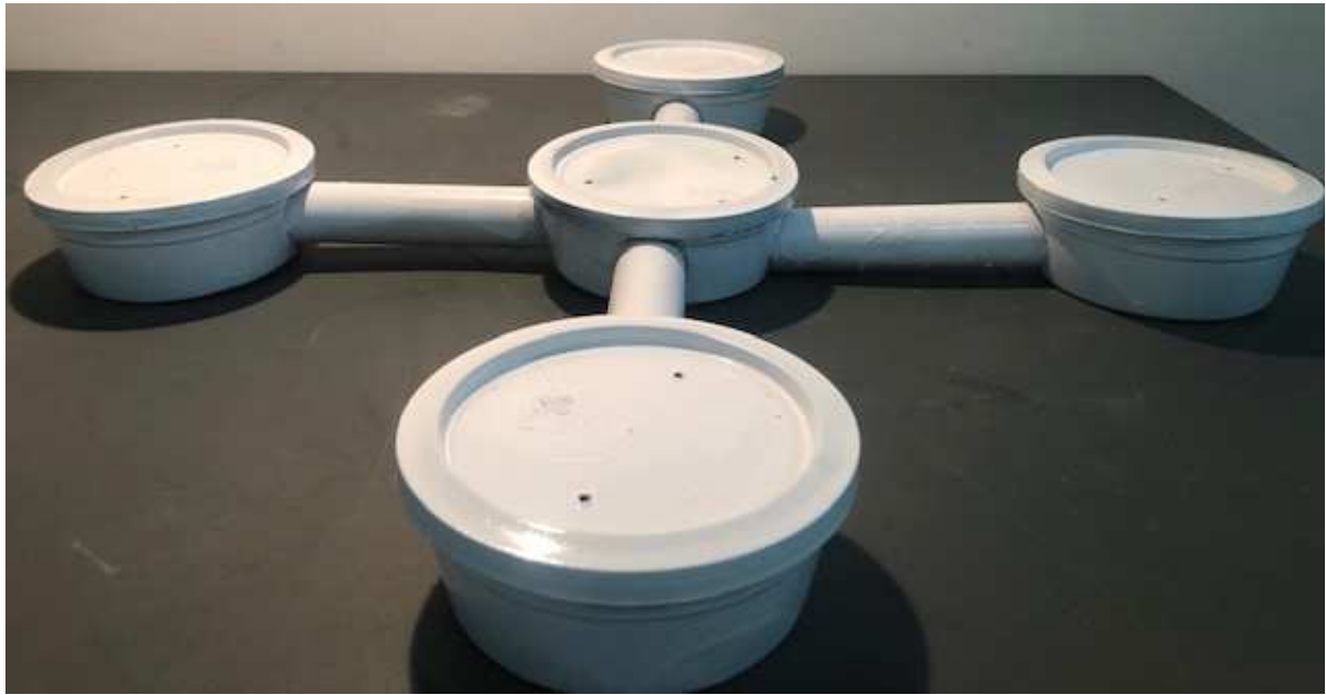
Figure 1. Four arms olfactometer used in this study.
