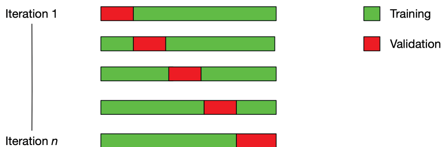
Figure 3.3. – Diagram of K-fold cross-validation, with k = 5 . Green and red squares represent subsets of data (i.e. folds) used for model training and validation, respectively.
