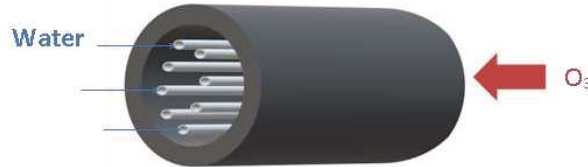
Figure 12. Configuration of membrane contactor with external/internal ozone transfer.
