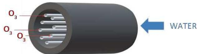
**Figure 11. Configuration of membrane contactor with internal/external ozone transfer.**
