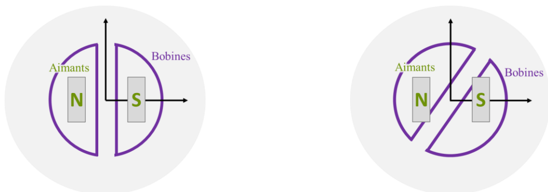
Figure 5 Illustration de l' Orientation Adjustable Path-type Magnetostrictive Transducers (OPMT) [Lee- et-al _2007]
