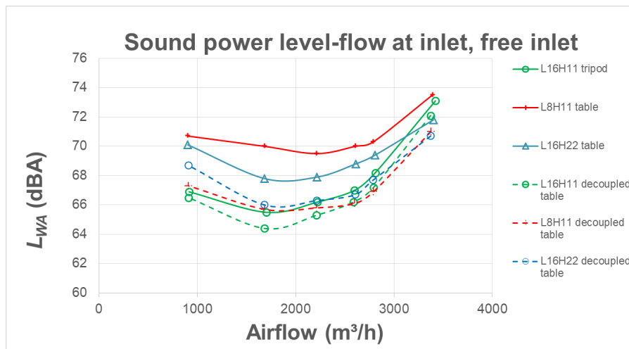
Figure B.4 – Sound power level at inlet for the serrated impellers with different assemblies
