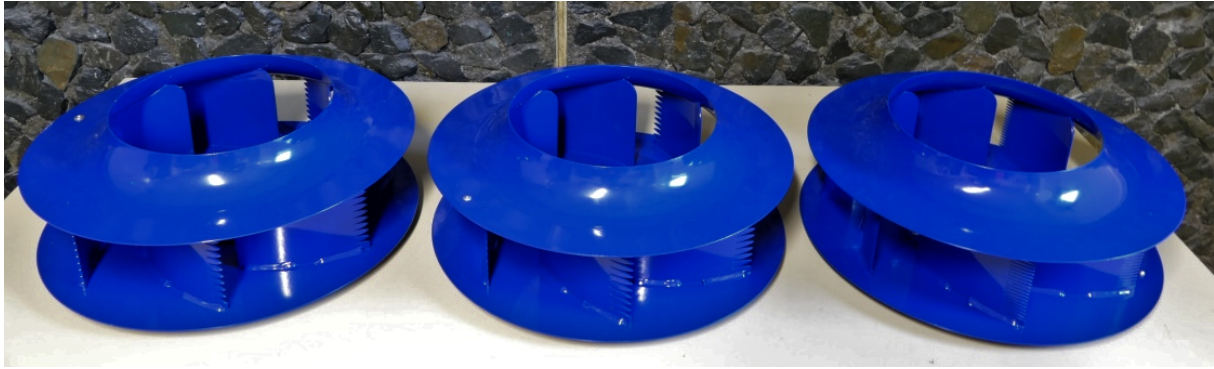
Figure 1.44 – Impeller prototypes with trailing-edge serrations
