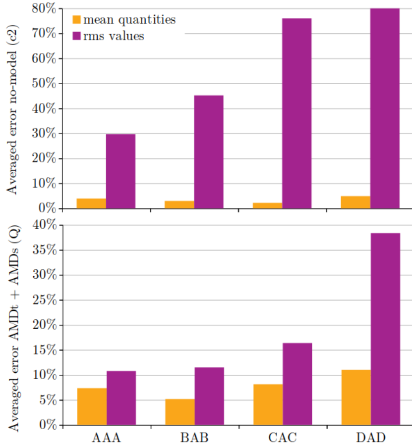
Figure 4.18 – Averaged errors obtained with four different meshes on mean quantities and RMS values. Simulations without model and with the tensorial AMD model are investigated.
