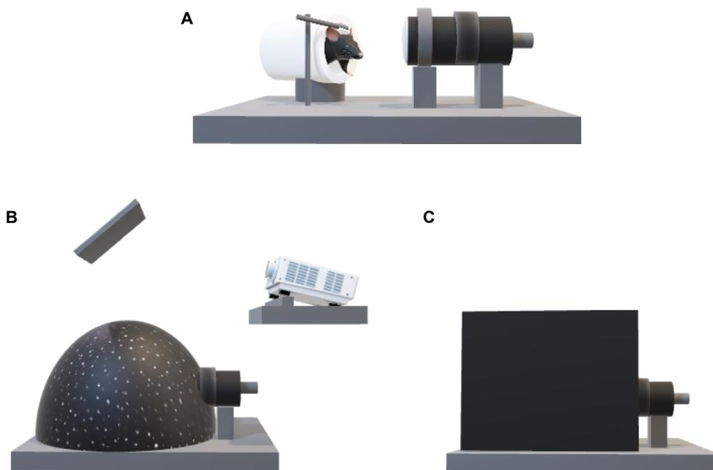
**Figure 27.** Visual and vestibular reflex tests. A- Mouse in turntable; B- OKR set up, with a dome surrounding the animal and a projector to induce optokinetic stimulation; C-VOR set up consisted in a box surrounding the animal and camera to completely isolate the animal and test the reflex in complete darkness. Credit Filipa FdB.
