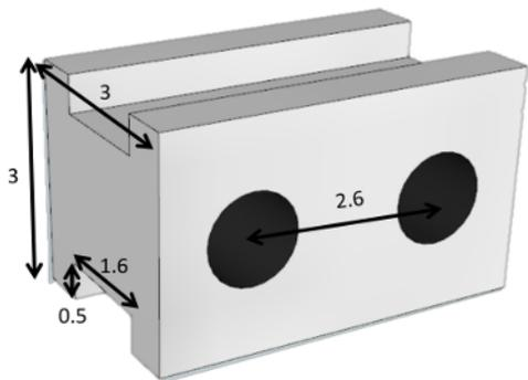
**Figure 2:** Headpost depicted with dimensions, in millimeters. Fixed in the implantation surgery, this light (0.2 g) poly (lactic acid) plastic headpost allows the locking of the adaptation device to the mouse and head-fixing of the animal on the turntable during the video-oculography sessions. [Please click here to view a larger version of this figure.](#)
