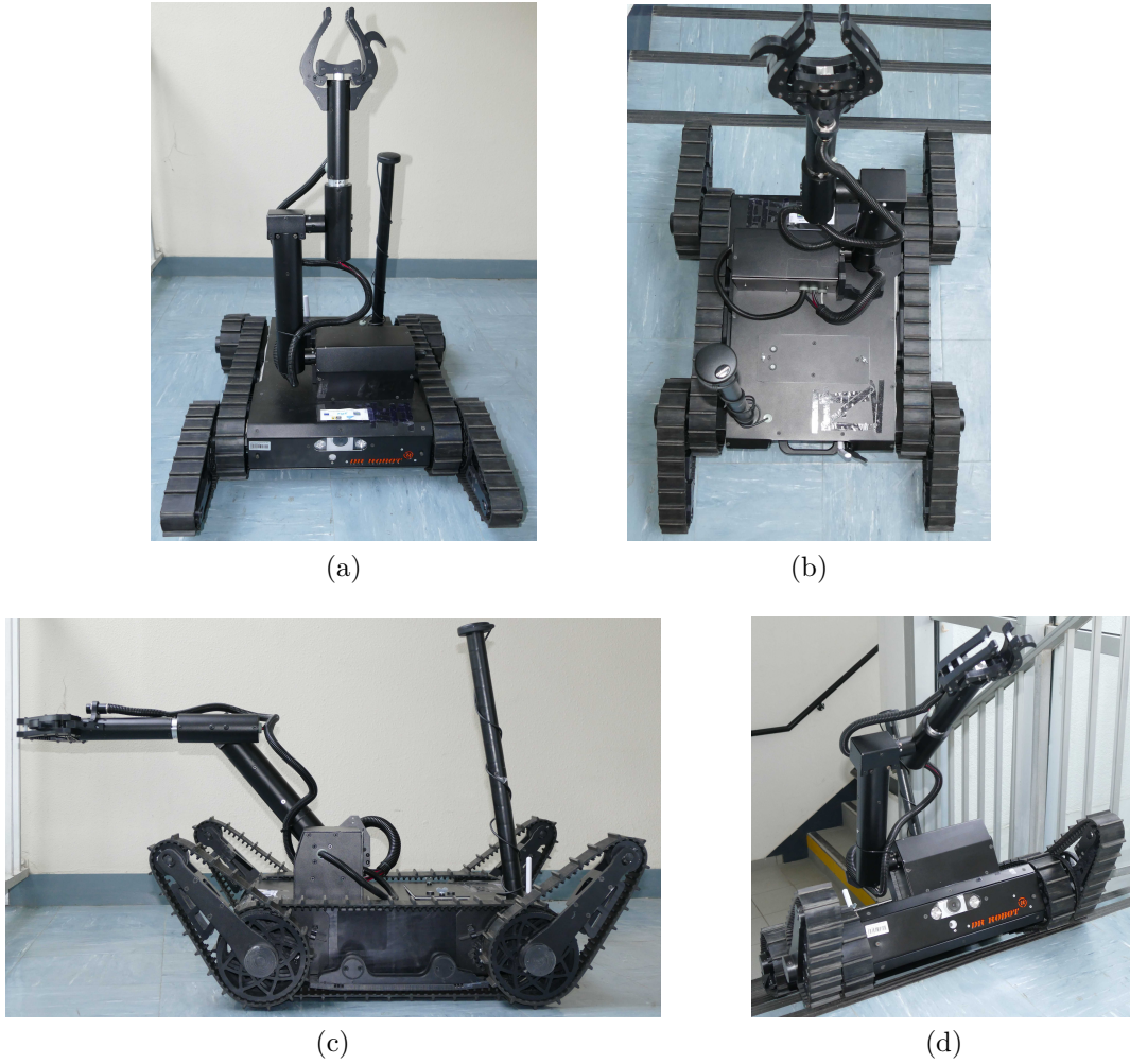
Figure 5.7: Jaguar in the "extended" configuration. Front view (a), top view (b), side view (c), "in-action" view (d)
