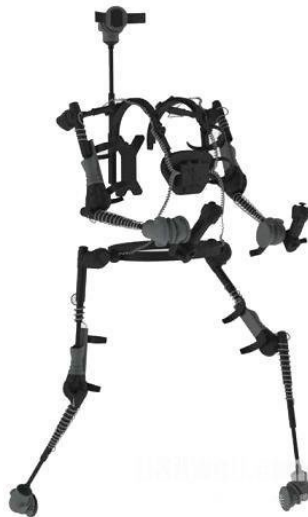
FIGURE 3.3: Example of the Gypsy 7 mechanical mocap system.
