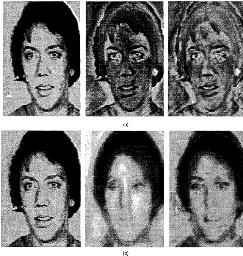
FIGURE 4.9: High-order eigenfaces carry accurate information for face recognition (O'Toole et al., 1993): (a) the original face (left), its reconstruction without using the first 20 eigenfaces (center) and without using the first 40 eigenfaces (right); (b) the original face (left), its reconstruction using only the first 20 eigenfaces (center) and using only the first 40 eigenfaces (right).
