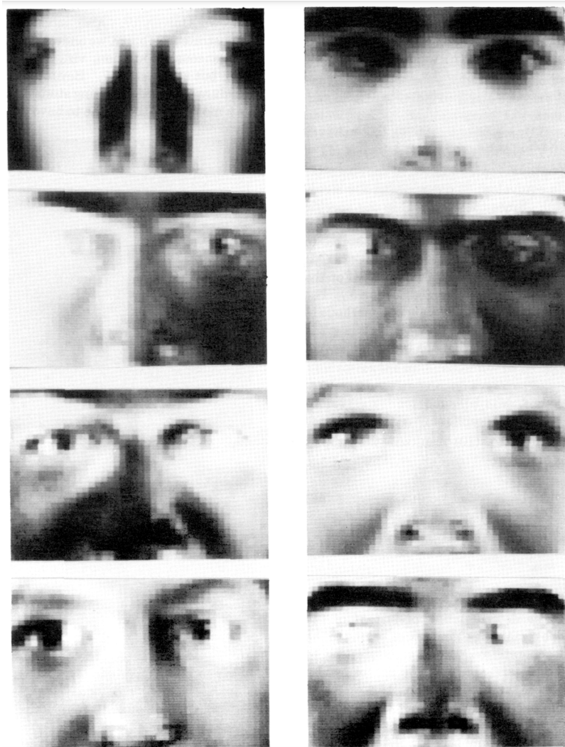
FIGURE 4.6: The first eight eigenfaces obtained from an ensemble of cropped grayscale face images in Sirovich and Kirby (1987) . Subfigures must be read from left to right, ending at lower right.
