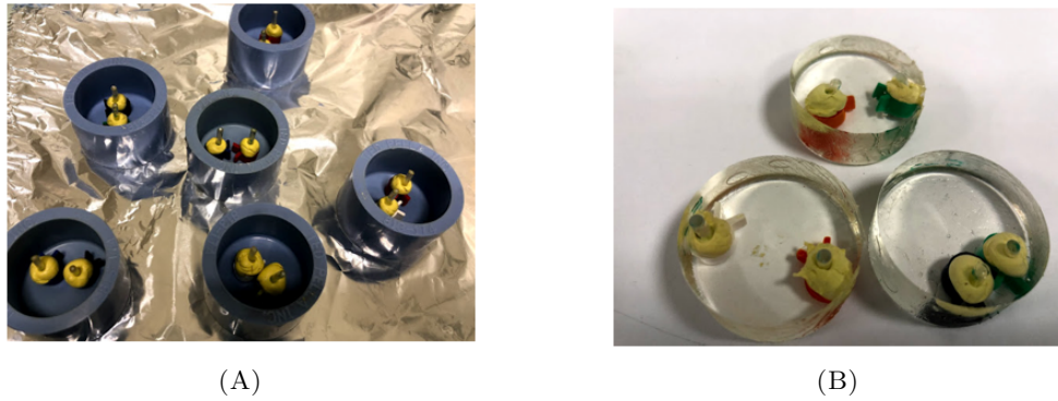
FIGURE V.10: Sample preparation with (A) installation of tubes in the mold and (B) demolded and polished samples
