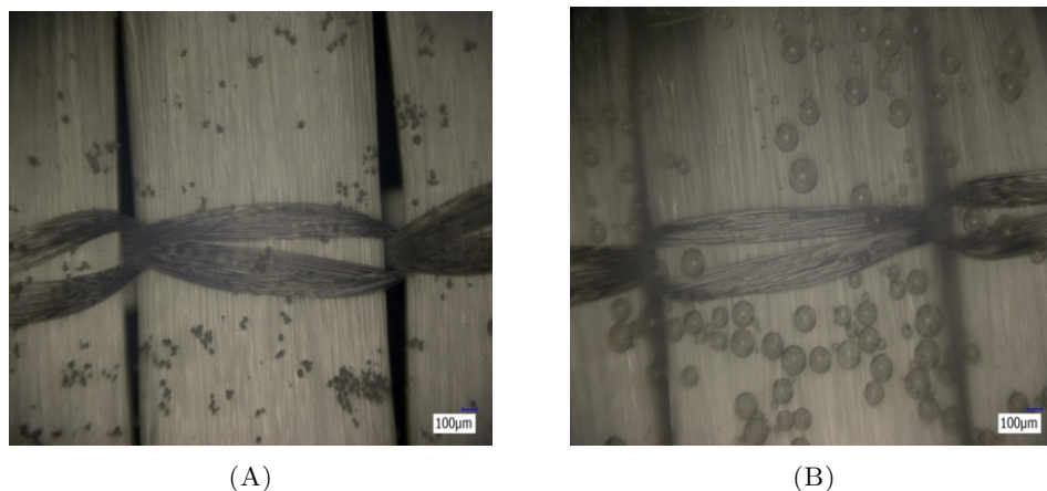
FIGURE III.3: Optical microscope images of Expancel particles deposited on the preform surface (A) before and (B) after heating
