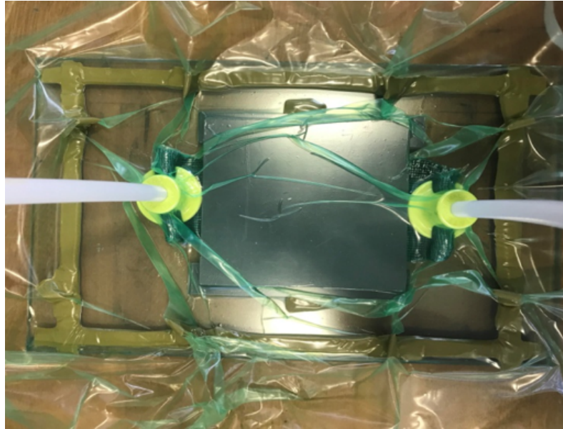
FIGURE III.17: Fabrication of functionalized composite panels using infusion between two plates
