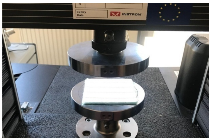
FIGURE II.3: Placement samples of the quasi-UD fabric within the compression platens of the universal testing machine Instron 5582
