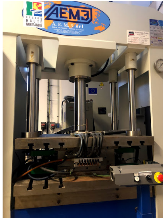
FIGURE III.1: An illustration of the induction machine constituted of a hydraulic press and the mold heated by induction
