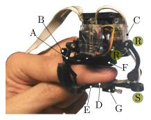
Figure 1: The Revolute-Revolute-Spherical fingertip device presented in [51].
