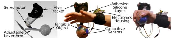
Figure 4: WeATaViX [58]. The device is composed of a 3D-printed static part anchored to an adhesive silicone layer attached to the hand. Two capacitive sensors cover the tangible object, respectively facing the palm and the fingers during grasp closure. The hands-on demonstration of this device won the Best Demonstration award at Eurohaptics 2020 and IEEE World Haptics 2021.
