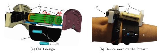
Figure 7: The proposed wearable device for the arm [53]. It consists of a static platform (A) that accommodates two servomotors (B) and two pulleys (C), a fabric belt (D), and four vibrotactile motors (E). The device is able to provide skin stretch, pressure, and vibrotactile stimuli to the arm.
