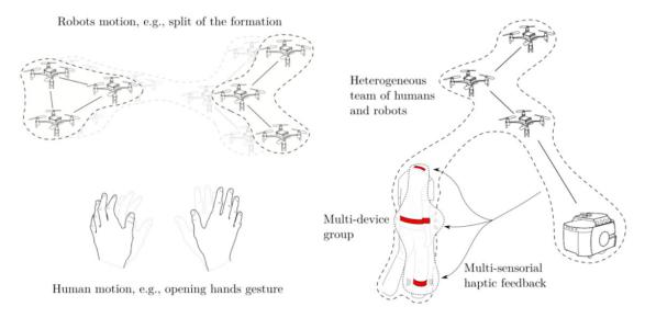
Figure 24: Representative scenario. (Left) A user controls the motion of six drones in a shared environment, splitting - with an opening-hands gesture - a connected team of drones in two so as to cover more ground. (Right) He receives vibrotactile and skin stretch feedback spread throughout the body - through a multi-device group, informing him about the status of the team(s), of the environment, and the task.
