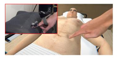
Figure 19: Use case from [43]. A human user wearing a finger device interacts with a tangible object that resembles the abdomen of a virtual human patient. Providing timely cutaneous stimuli via the wearable haptic device, we can alter the stiffness and shape perception of passive tangible objects. For example, in the context of medical palpation, we can simulate the presence of a tender bodypart or of a small bump representing a cyst.
