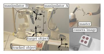
Figure 8: Haptic-enabled shared control enables one operator to control a robotic system composed of two arms. [15].
