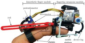
Figure 2: The combined kinesthetic-cutaneous device presented in [54].
