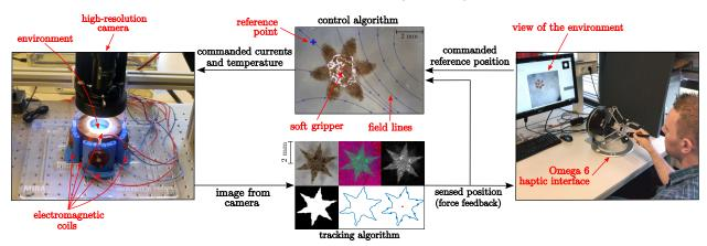
(a) Interconnected haptic-enabled micro teleoperation system.
