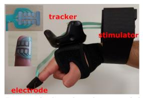
Figure 18: An electrical stimulator is attached to the forearm and the electrode is placed in contact with the finger pad. The user's hand is tracked by a HTC Vive Tracker [138].
