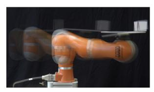
Figure 10: A teleoperated robot manipulator transports an object grasped in a nonprehensile configuration while autonomously modulating the user-specified inputs and the object orientation to prevent it from sliding and possibly falling under the action of gravity [89].
