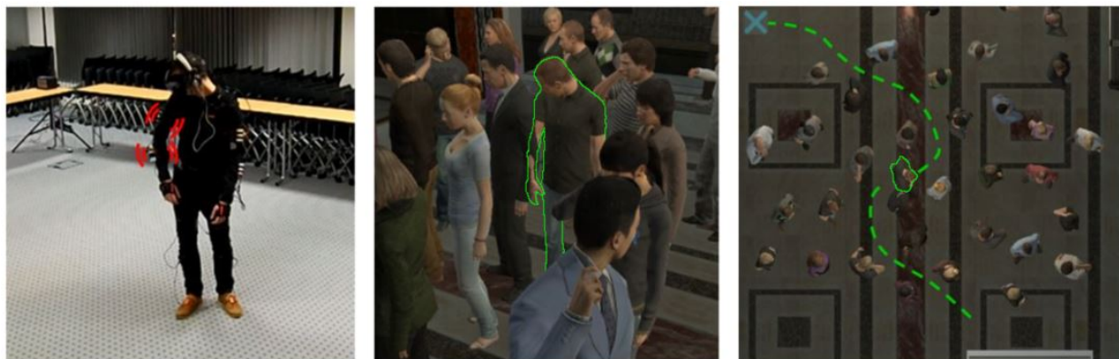
Figure 21: The objective of [30] is to understand whether and to what extent providing haptic rendering of collisions during navigation through a virtual crowd (right) makes users behave more realistically. Whenever a collision occurs (center), armbands worn on the arms locally vibrate to render this contact (left).
