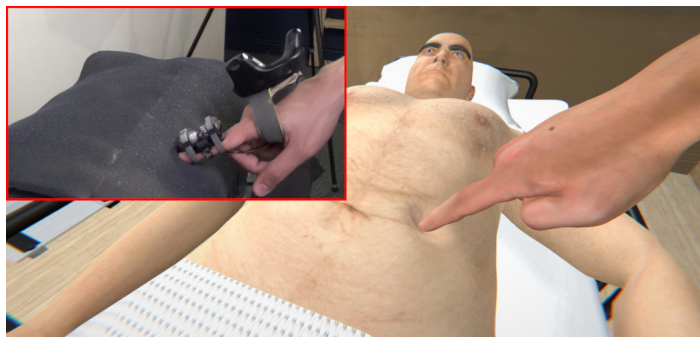
Figure 19: Use case from [43]. A human user wearing a finger device interacts with a tangible object that resembles the abdomen of a virtual human patient. Providing timely cutaneous stimuli via the wearable haptic device, we can alter the stiffness and shape perception of passive tangible objects. For example, in the context of medical palpation, we can simulate the presence of a tender bodypart or of a small bump representing a cyst.
